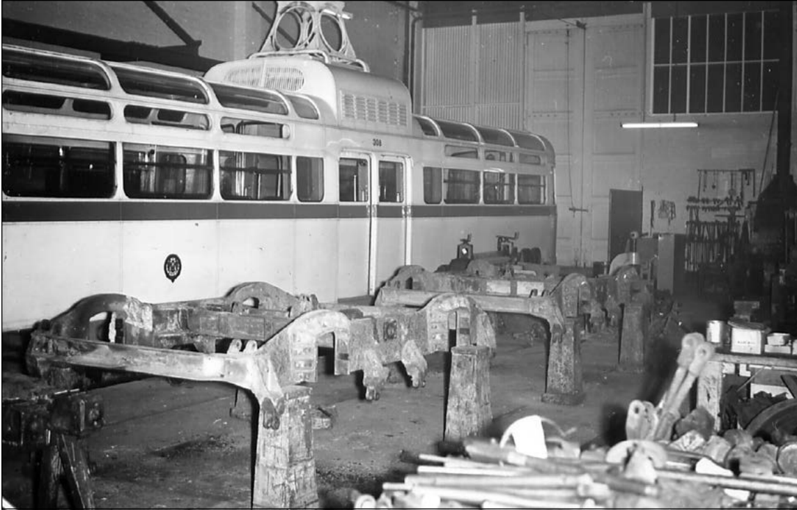
Coronation 317 in the Fitting Shop over the wheel drop pit, with EE bogie frames in the foreground, ready for cleaning and repainting in January 1964. (Author)
