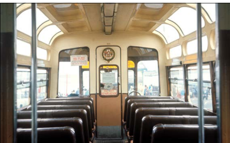
(Left) The bright spacious saloon of a Coronation with fling-over seats, seen at the Fleetwood terminus. (Right) The saloon of 310 with the 64 bus seats facing in opposite directions on each side of the aisle.
