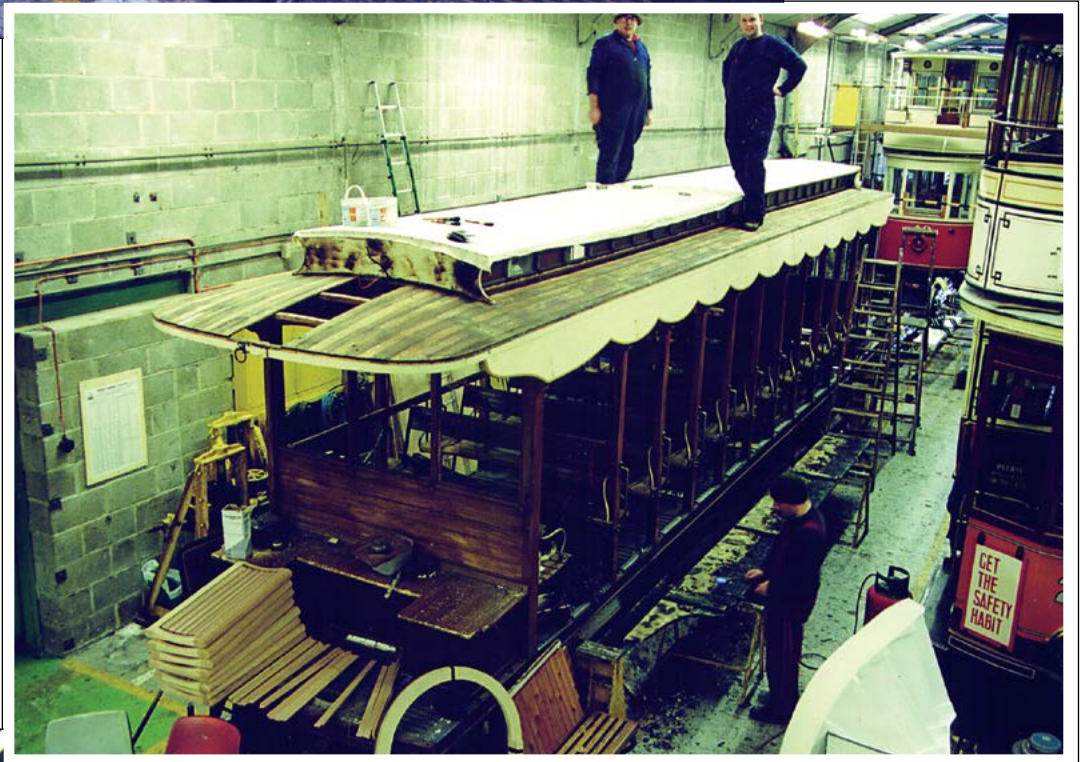
(Centre) New grooved boards have been fitted, and new canvas applied to the raised centre section of the roof. Seats and body-frame have been varnished.
