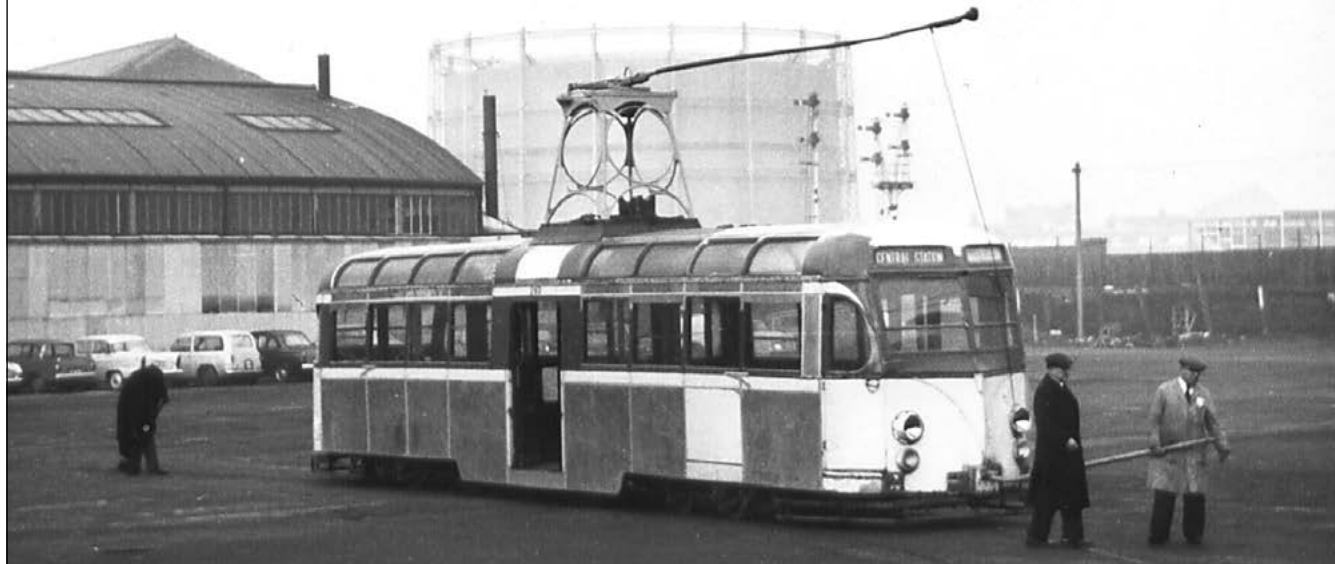
In January 1964, Railcoach 269, later OMO 1, having been repanelled in the Body Shop, is about to be shunted into the Paint Shop. This view shows the traverser and the old Works, now the Bus Park. (Author)
