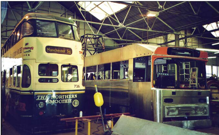
In January 2006, 648 has had new panelling fitted, and been joined by 726 being fitted with new saloon flooring. The Centenary car is keeping its 1985 front appearance, and the new higher facia roof-panels are tapering down to the indicator. The front has been modified, making it lower than originally, and thereby replacing the lifeguards. (Author, both)
