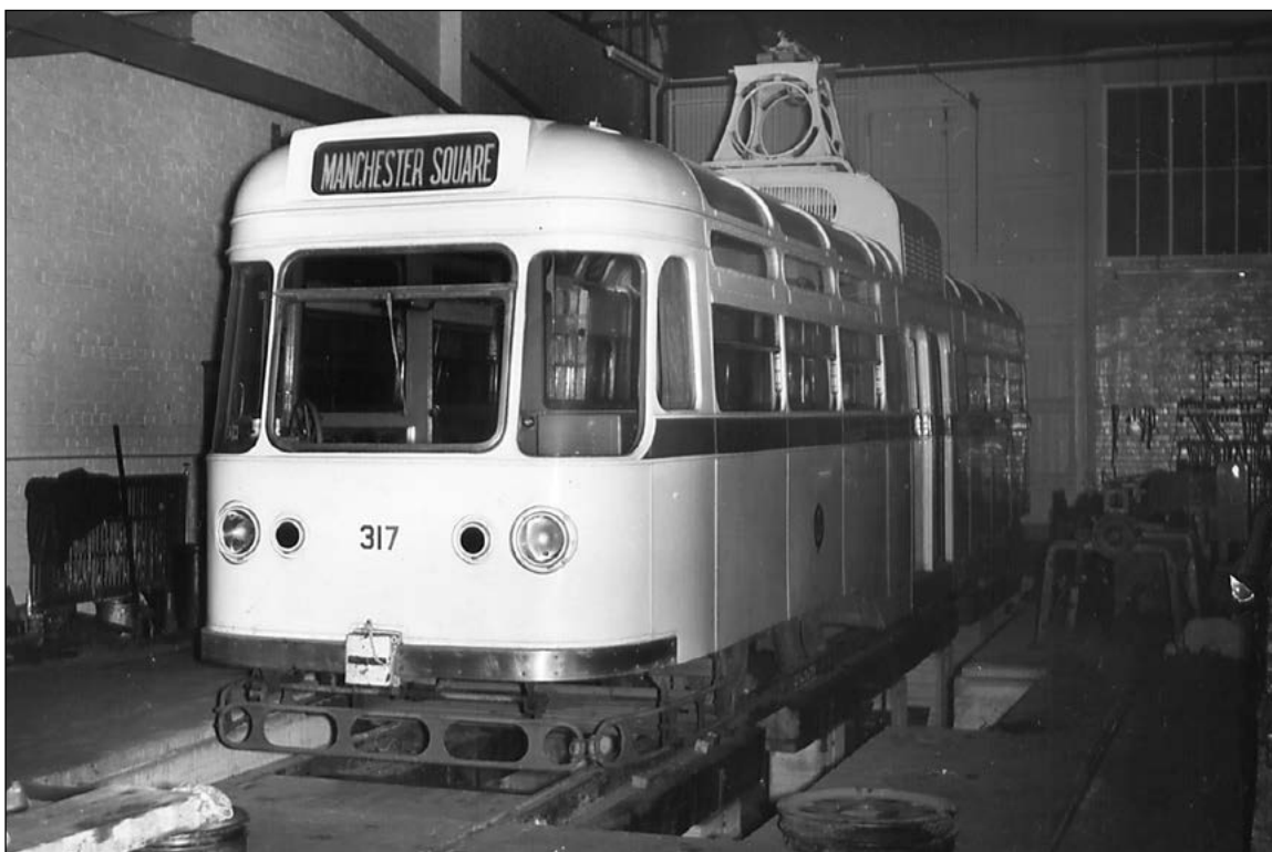
Coronation 317 over the wheel-drop pit and a detached wheel in the foreground. (Author)
