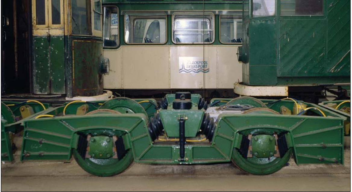
View of the Metalastik bogies for 762 and Centenary cars, showing the rubber inserts for the axle-boxes and the longer bogie-frame. (Author)
