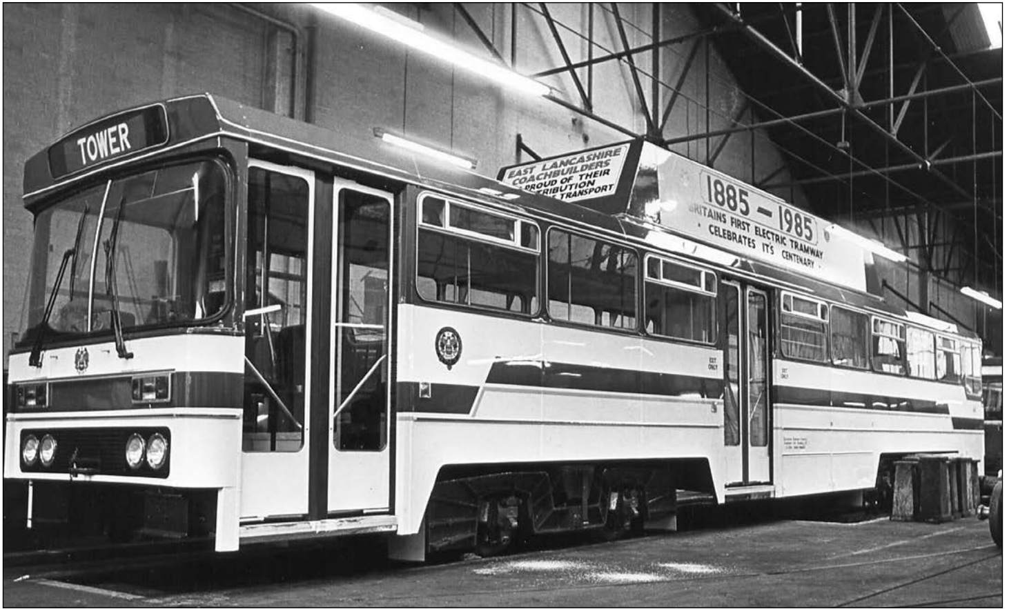
In the Fitting Shop, 641 has been mounted on its new bogies. Though it has not yet gained its pantograph tower, it still looks handsome. ( The Gazette )
