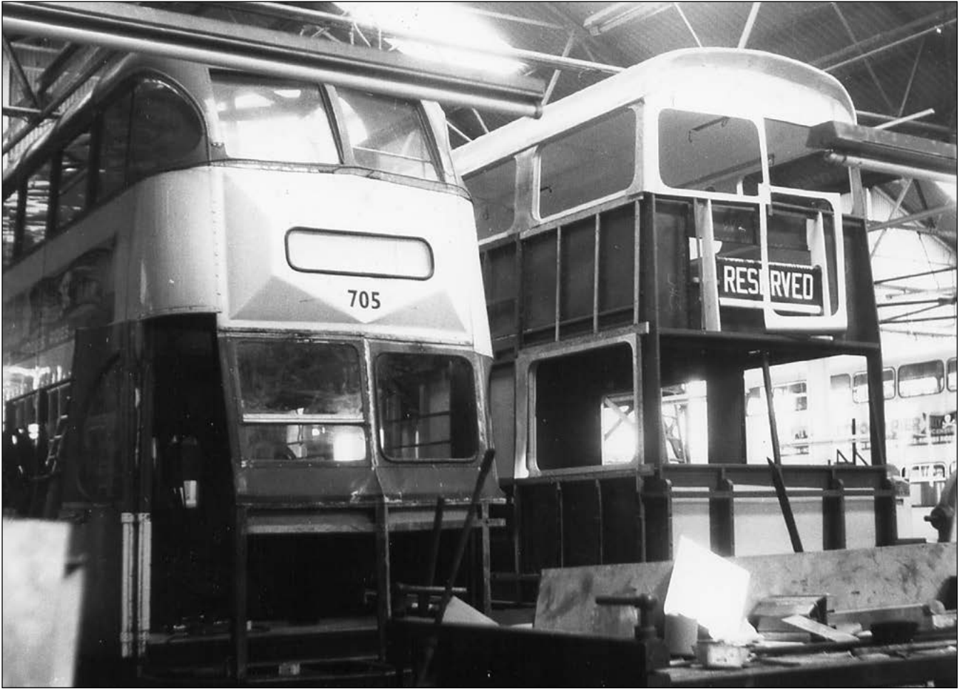
(Above) A contrast in appearance between 705 and 761, seen undergoing rebuilding in the Body Shop during 1978. The new end-section frame is impressive.
