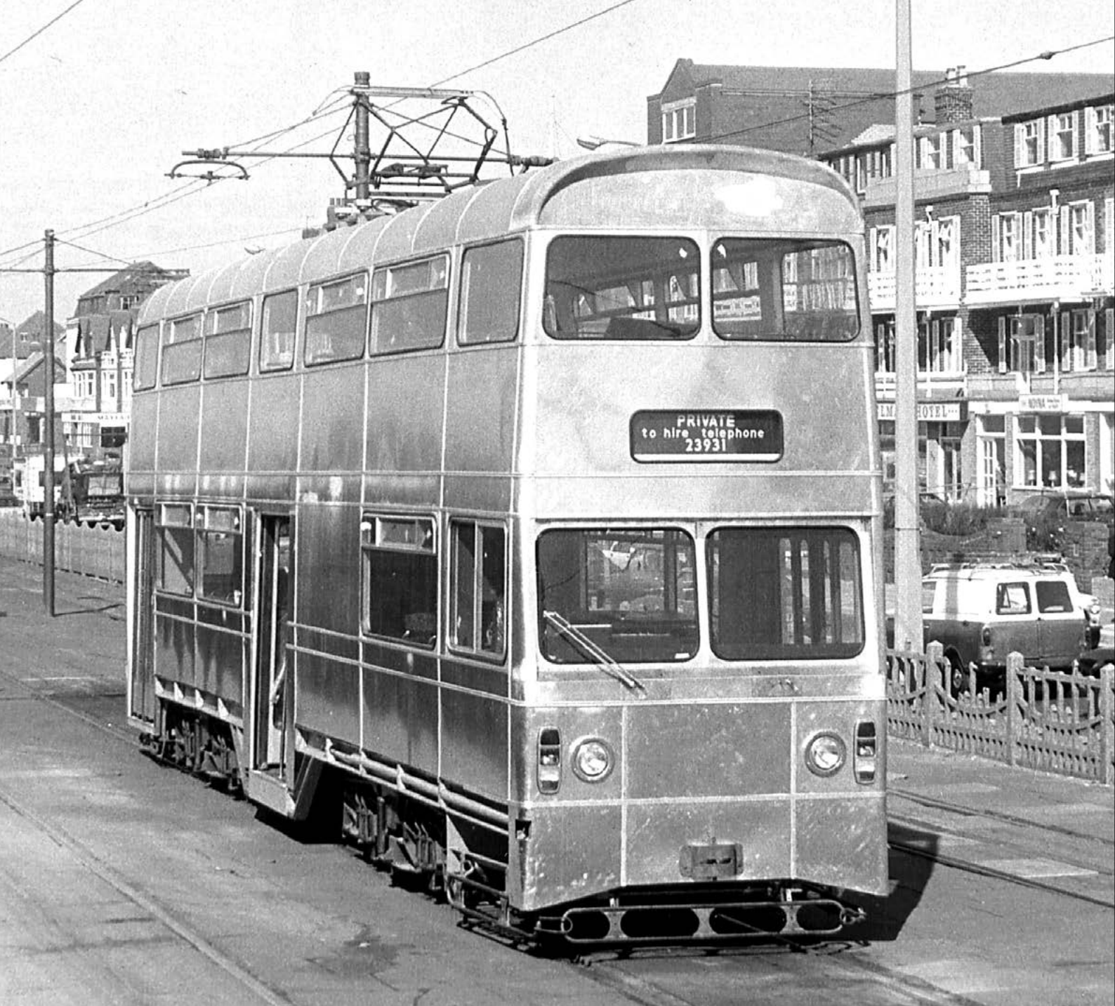
Number 762 on its first trial run at Bispham on 1st April 1982, unpainted and showing the bogies without the lower panelling, in order to test their clearance on curves. The peaked domes replicate contemporary bus design fashion. (Author)
