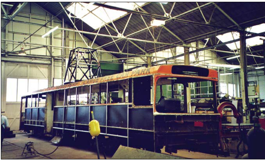
October 2005 and 648 is seen, above, in the Body Shop, with the body panels removed. Notice the original-style tower has been restored.
