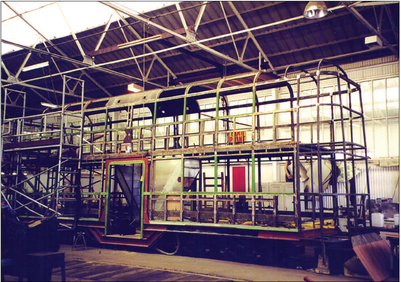
The complete body-frame of 718 seen in the Body Shop during August 2000, the original teak frame having been extended by a metal frame in the new style. (Author)
