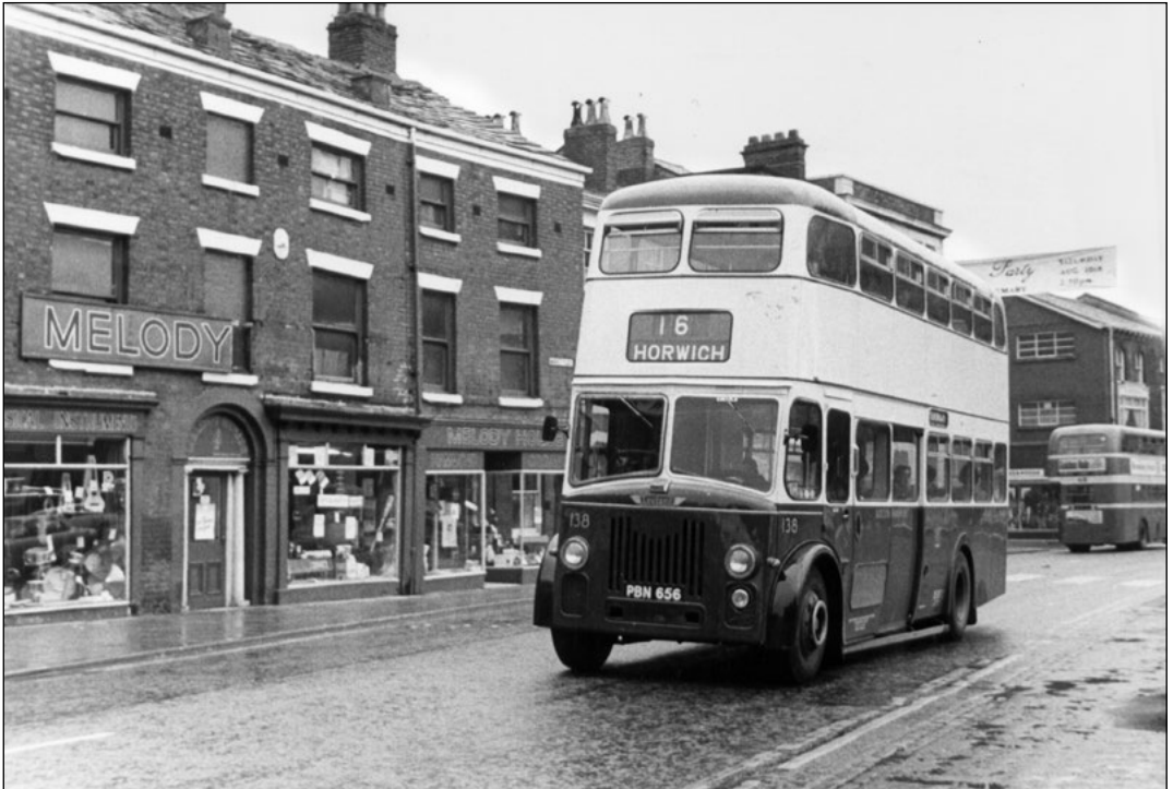
Two Leyland PD2s, both with Metro-Cammell bodies, but showing contrasting styles. In the upper photograph No. 125, dating from 1957, has traditional radiator and rear entrance open platform bodywork, which was the 'norm' for British double-deckers for many years. The lower photograph shows No. 138 dating from 1961, only two years later but with full front, concealed radiator and front entrance body. In the distance one of Ribble's large fleet of Leyland double-deckers moves away from the camera. (BD both)
