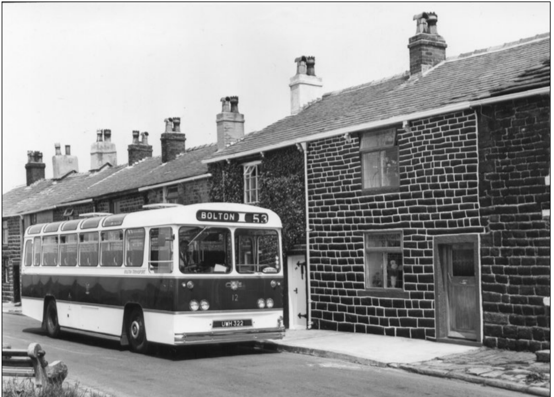
The first single-decker to be received since 1956 arrived in 1962 and was an East Lancashire Coachbuilders-bodied Leyland Leopard L2 with fleet number 12. It had dual-purpose high-back seating for 41 passengers together with curved glass cantrailis. It is shown above on more mundane duties leaving Moor Lane Bus Station for Affettside, and followed by a Leyland PD2/4 still in the maroon-and-three-cream-bands livery which now looks very dated by comparison with the Leopard. In the lower view at the other terminus the era of renovation and upgrading of the old cottages has clearly begun. ( BD, STA courtesy BCVM ).
