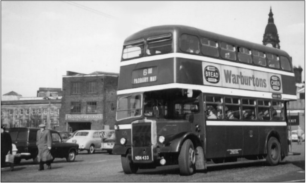
The year 1959 also saw a return to 27ft long double-deckers with the purchase of five Leyland PD2/37 models with Metro-Cammell bodies. Number 125 illustrates this batch as it leaves Moor Lane Bus Station in April 1962. (RM)
