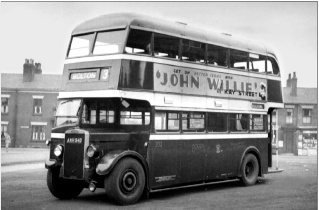
Another example of an East Lancashire Coachbuilders body supplied in wartime is shown fitted to No. 202, dating from 1941. The body, which was supplied in 1945, was originally fitted to 1936 Leyland TD4c No. 34. (RM)
