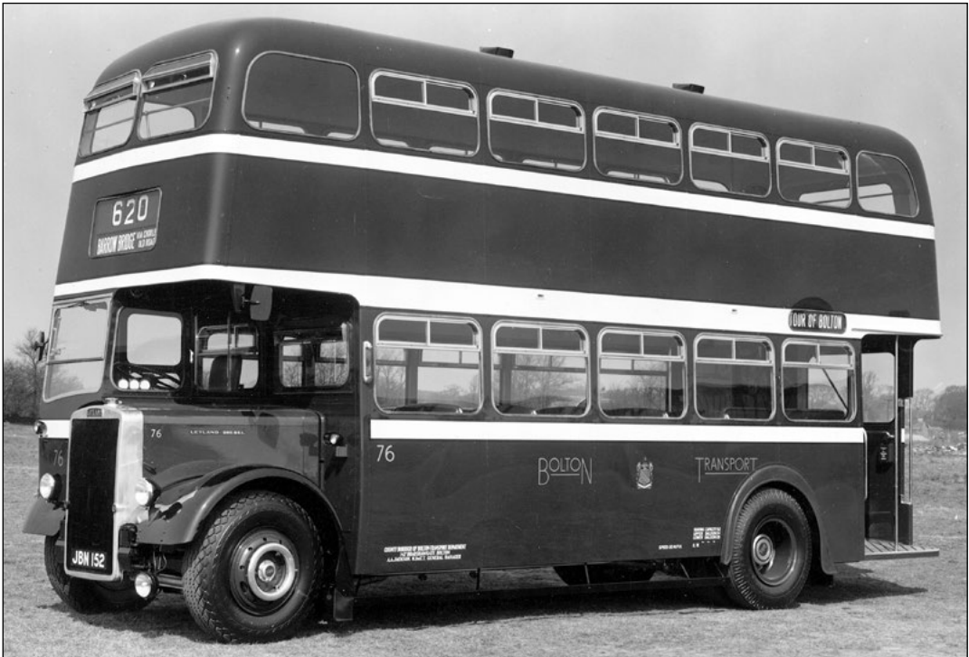
The other double-deck deliveries in 1956 were nine Metro-Cammell bodies, also on Leyland PD2/13 chassis, and numbered 76-84. The first of the batch was photographed before delivery from Birmingham when new. (STA)
