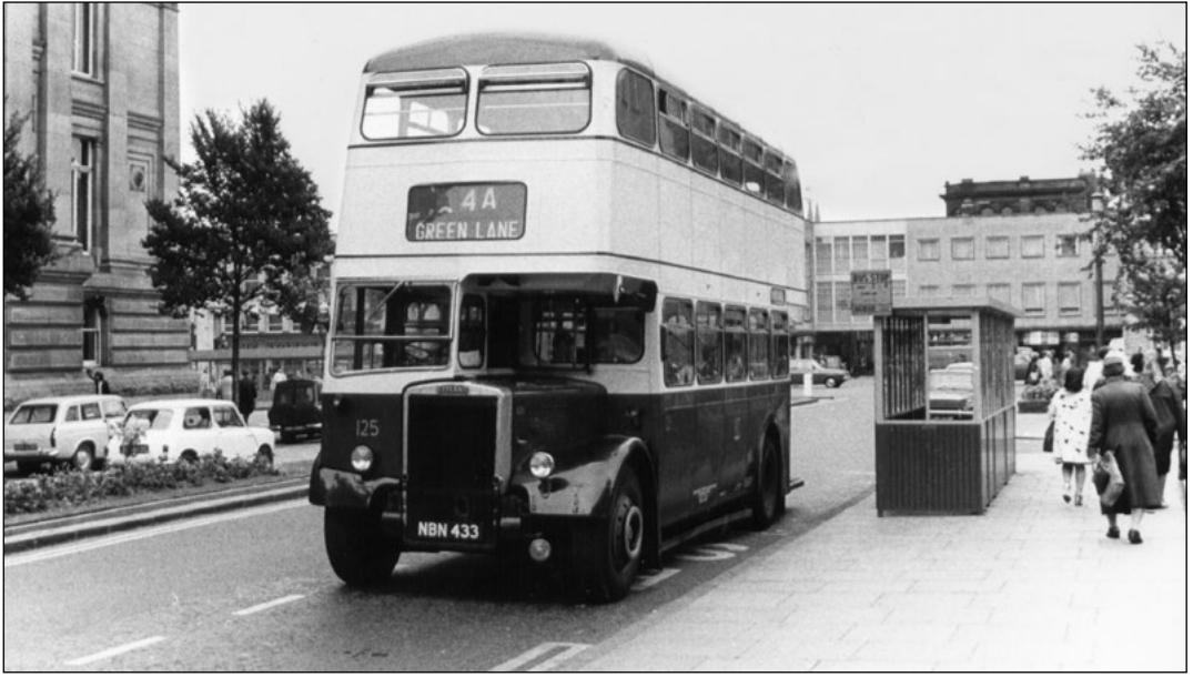
Two Leyland PD2s, both with Metro-Cammell bodies, but showing contrasting styles. In the upper photograph No. 125, dating from 1957, has traditional radiator and rear entrance open platform bodywork, which was the 'norm' for British double-deckers for many years. The lower photograph shows No. 138 dating from 1961, only two years later but with full front, concealed radiator and front entrance body. In the distance one of Ribble's large fleet of Leyland double-deckers moves away from the camera. (BD both)
