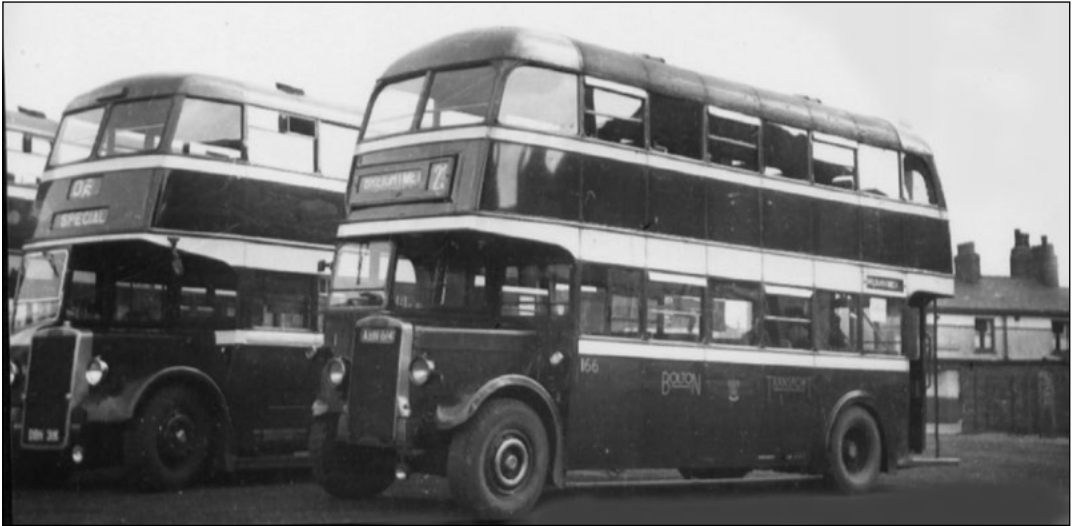
Above: Number 166 from the 1939 delivery of Massey-bodied Leyland TD5c models was still looking quite smart when photographed 10 years later in September 1949, alongside a recently delivered Leyland-bodied Leyland PD2 No.416. (RM)
