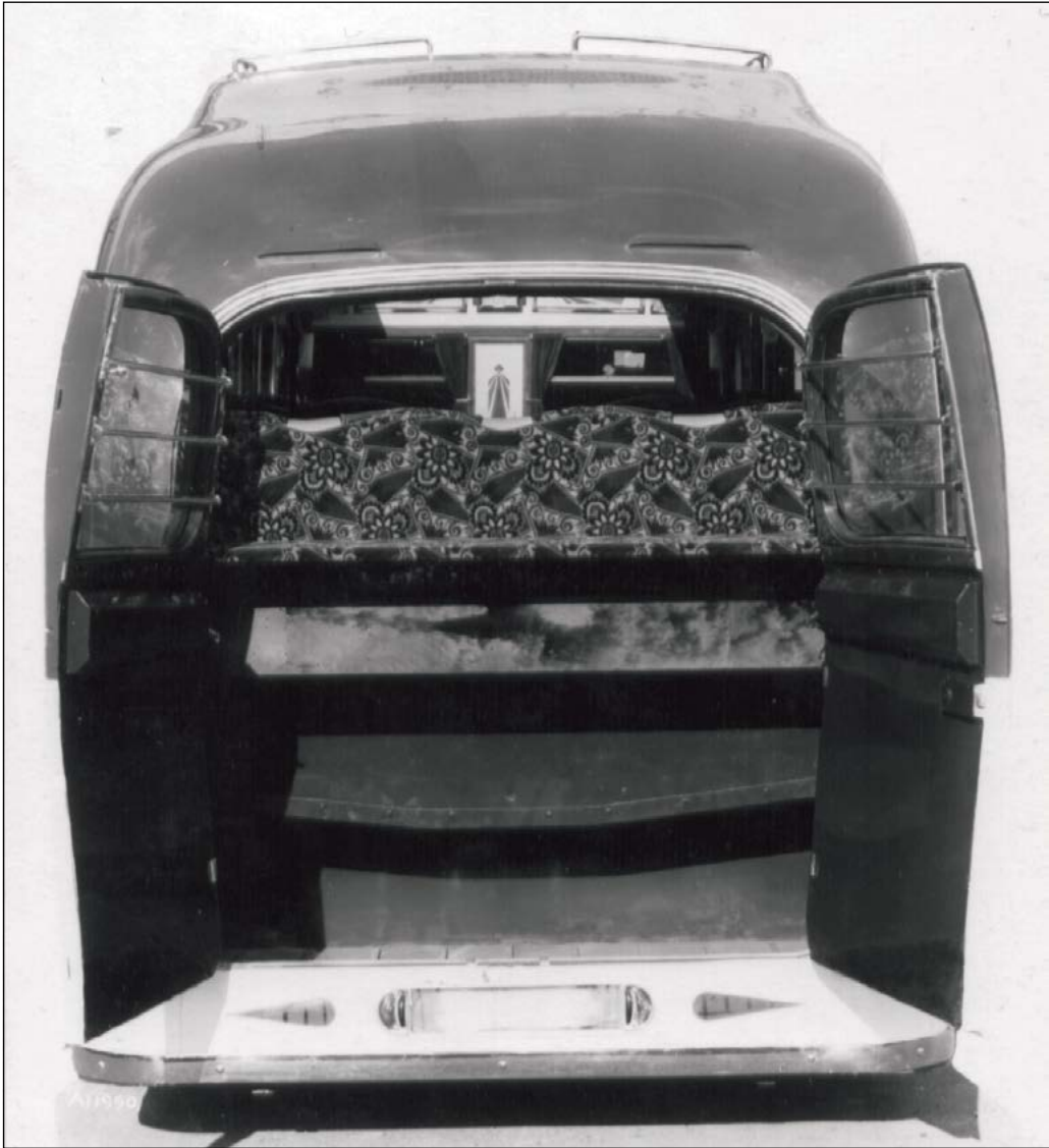
Returning to the previously mentioned problem relating to the accommodation of luggage, Red & White's solution was the fitting of full depth doors at the rear of the coach to access the luggage compartment, which was still at this stage supplemented by a roof rack. (STA)
