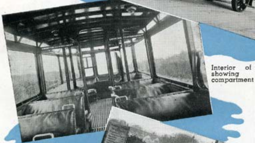
1920. A.E.C. "B" type (note windows open and close) The first attempt at adjustable windows.
