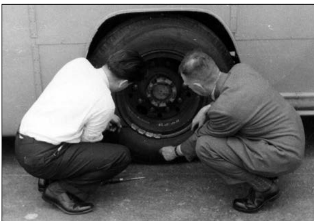
Tyres needed to be thoroughly examined after each test drive of the Midland Red CM5 (R.E.S. Richards/Midland Red Coaches collection)
