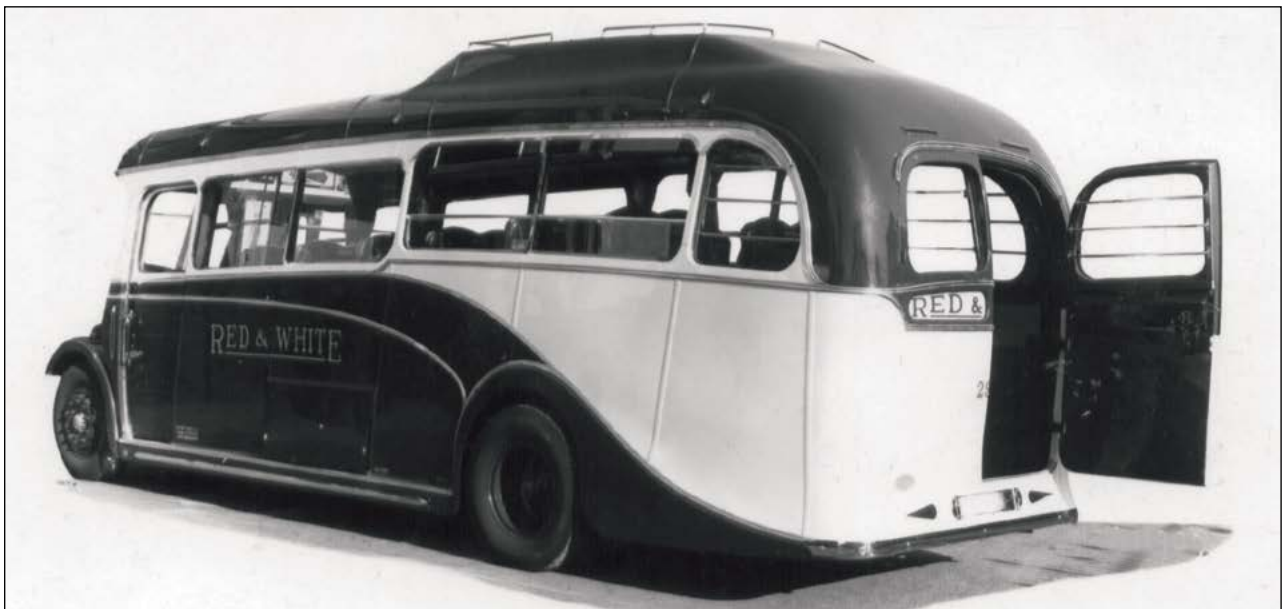
Returning to the previously mentioned problem relating to the accommodation of luggage, Red & White's solution was the fitting of full depth doors at the rear of the coach to access the luggage compartment, which was still at this stage supplemented by a roof rack. (STA)
