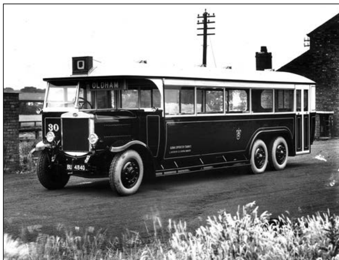
Number 30 (BU 4840) was a forward-control Guy FCX with a 39-seat Roe body delivered in 1927. It lasted for eight years and later became a caravan at Moorside. (STA)
