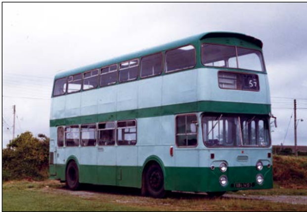
Above. Number 460 (PBU 960), a Leyland PD2/30 with Northern Counties body, was delivered to Oldham in January 1959. It became SELNEC 5360 and was withdrawn in 1971 and sold to Paton of Renfrew, in whose colours it is pictured. (JJH)
