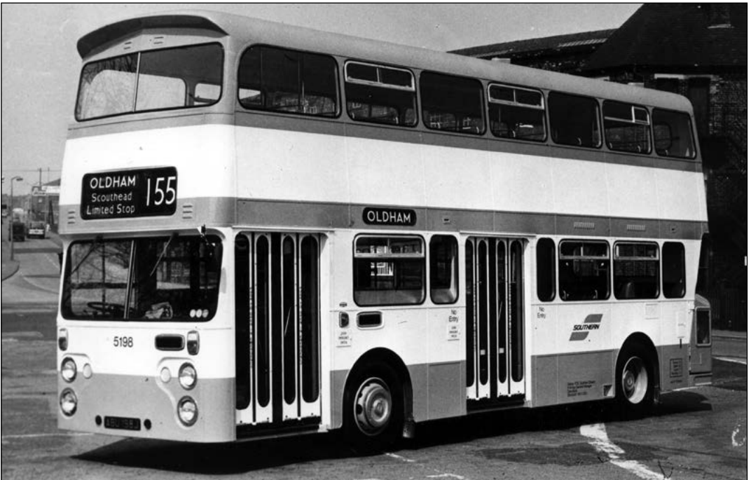
17 Roe-bodied Leyland Atlanteans were delivered to Oldham after the takeover date. Number 5198 (ABU 198J), numerically the penultimate Oldham bus, arrived in 1971 in full SELNEC orange livery. It is seen here posed outside the depot on arrival. (JJH)
