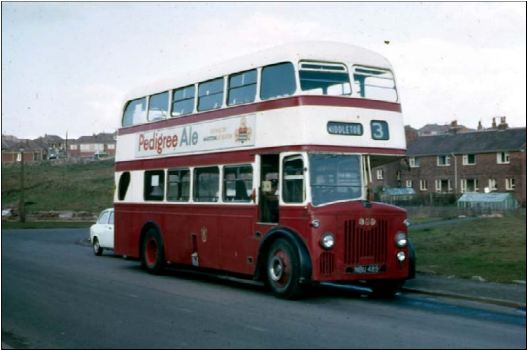
Thirty-one Leyland PD2/20s were delivered during 1957 carrying a mix of Roe, Crossley and Northern Counties bodies. Two of the Roe versions are shown here. In the upper picture number 389 (NBU 489) waits at the Rushcroft terminus of service 3 when new while below number 391 (NBU 491) stands in Car Street, between the workshops and the depot, after its withdrawal from service in 1973 and subsequent transfer to driver training duty as SELNEC's TV3. (both JJH)
