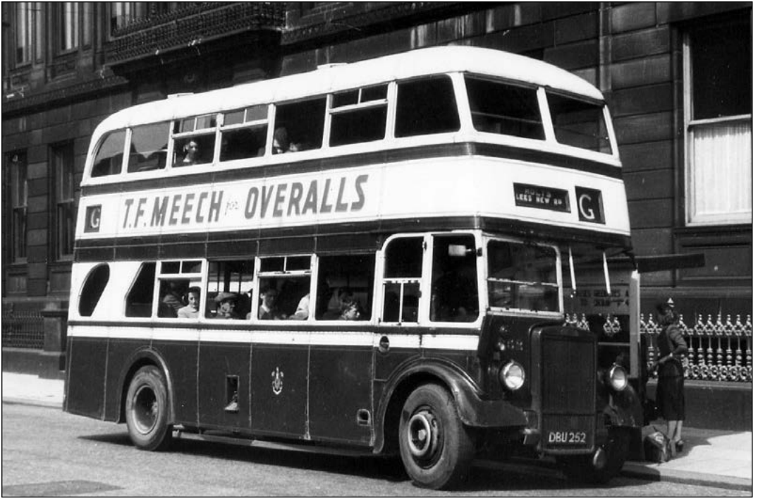
Oldham was quick to take advantage of the new regulations permitting 8ft wide buses and in 1947 took delivery of 25 Roe-bodied Leyland Titan PD1/3 models, the wider version of the PD1. Number 252 (DBU 252) is pictured on Union Street on service G to Abbey Hills. (MMT)
