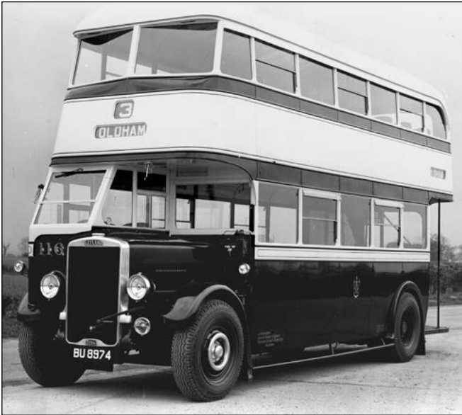
Centre. By comparison number 116 (BU 8974) looks far more modern with its experimental Roe 5-bay metal-framed body. It lasted longer than most of its contemporaries, being withdrawn in 1950 and passing to a showman. (STA)
