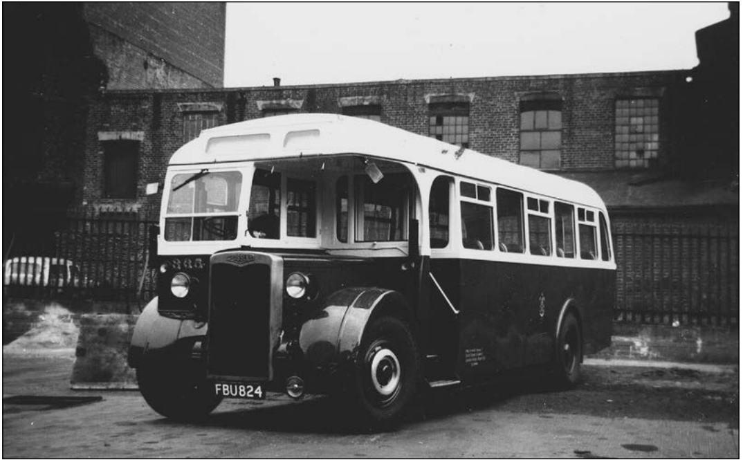
Number 365 (FBU824) was the last of four Crossley SD42/7 chassis fitted with Crossley bodies which were delivered in 1950 and saw off the last of the pre-war single-deckers. It is pictured in the depot yard at Wallshaw Street. Note the generally more solid appearance than Roe-bodied number 293. (STA)
