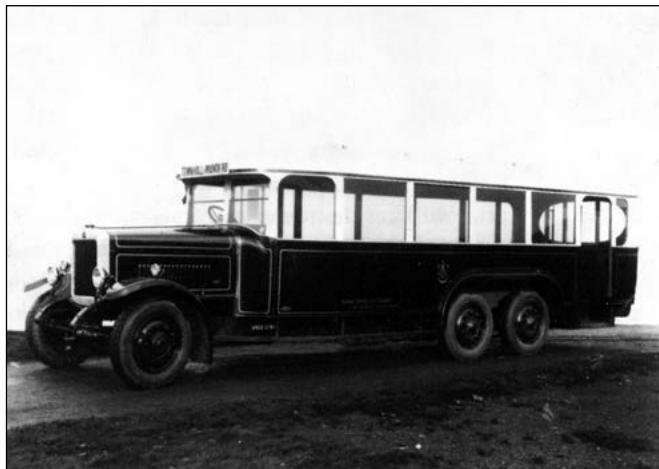
More conventional than the three double-deckers was number 22 (BU 5475), a basically similar BKX chassis but fitted with a single-deck body. Delivered in 1927, 22 was one of those taken by Leyland in 1934 in part exchange for new buses. (STA)
