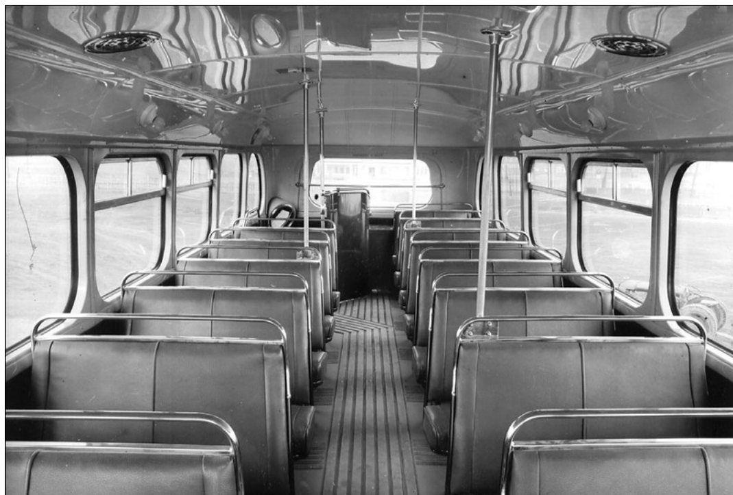
The interior views of the Burlington trolleybus bodies show attractive moquette seating in the lower saloon and brown Rexine-covered seats in the upper saloon, moquette not being considered appropriate in an environment where smoking was still customary. (GMTS)
