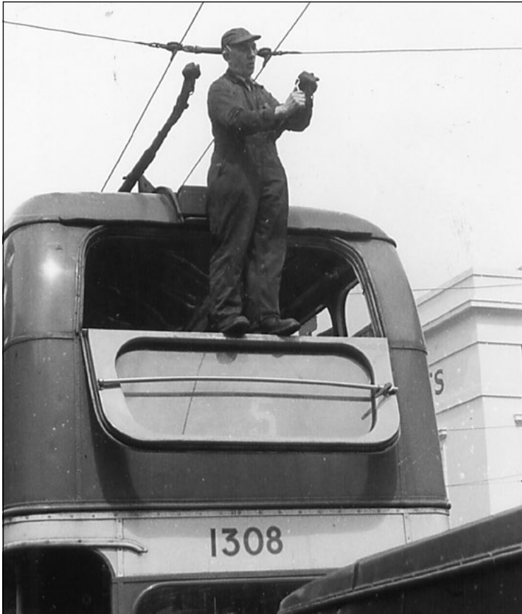
In today's safety critical industrial climate, such a scene would be unthinkable. But if a tower wagon was not handy, the only way to inspect and repair trolley heads was to use the emergency door at the rear of the upper deck. Some operators specified a solid panel in the emergency exit in order to provide a safe working platform for the linesman or fitter. (STA)
