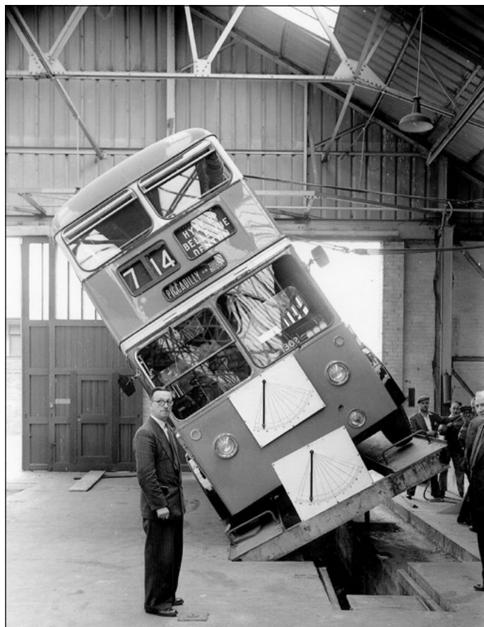
Manchester's first BUT, with body by HV Burlingham of Blackpool, was delivered in the summer of 1955. Here, the vehicle in question, No. 1302, is shown meeting the requirement to tilt successfully to 28 degrees in a decidedly more sophisticated environment than the earlier Crossley views with blocks of wood and jacks being used to raise the vehicle. Manchester was already buying motor bus bodies from the Blackpool factory though there had been questions about the use of non-union labour and other related issues which had needed to be resolved before the contracts could be confirmed. (RGRC)
