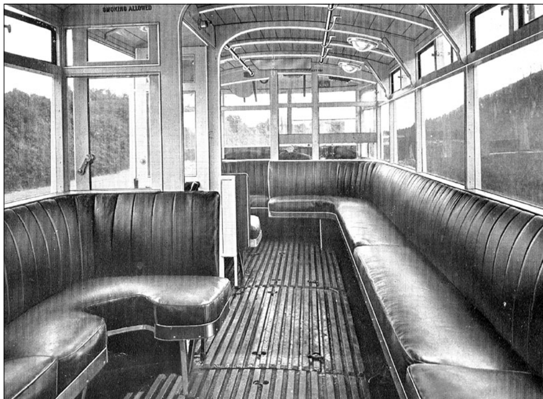
Six of the Railless trolleybuses delivered to inaugurate Ashton and Olham's first service were fitted with longitudinal seating as seen above; the other four had a mix of longitudinal and transverse, the seating capacities being 36 and 37 respectively. (GLC)
