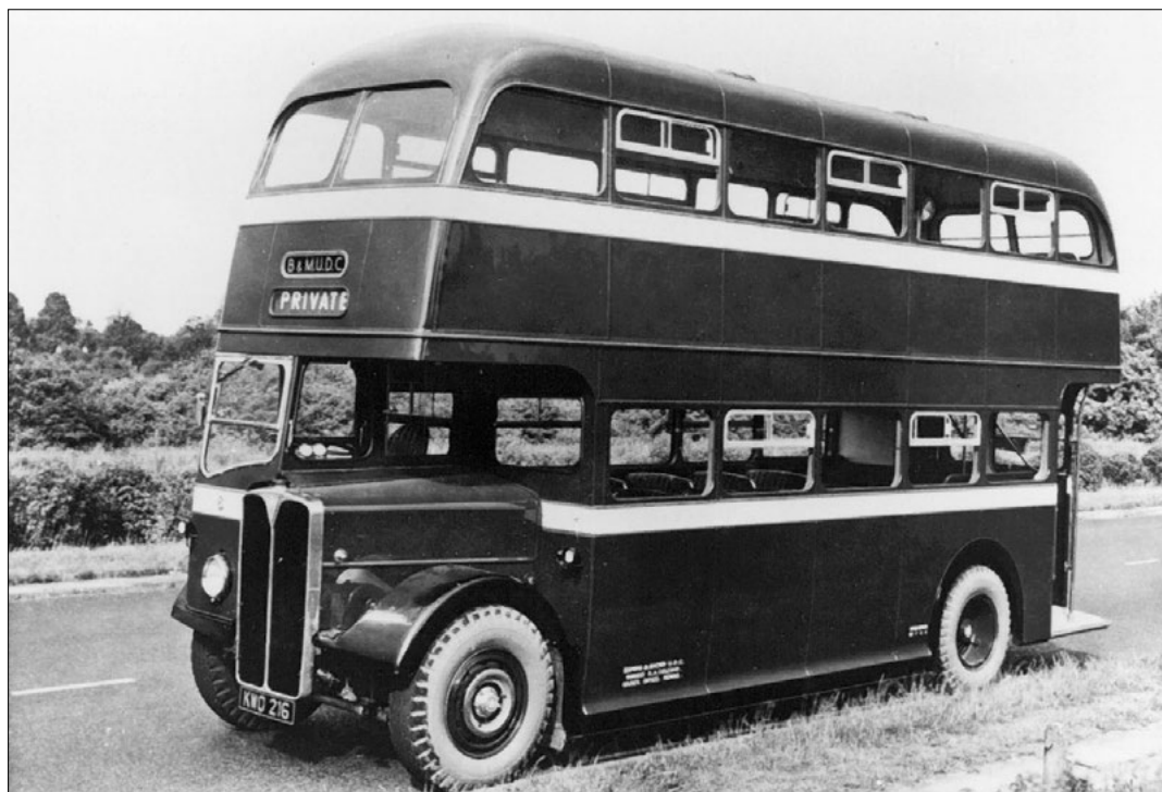
The only highbridge double-decker ever owned by the Council was AEC Regent III KWO 216, numbered 8, built with a series for Aberdare with handsome Northern Counties bodywork.
