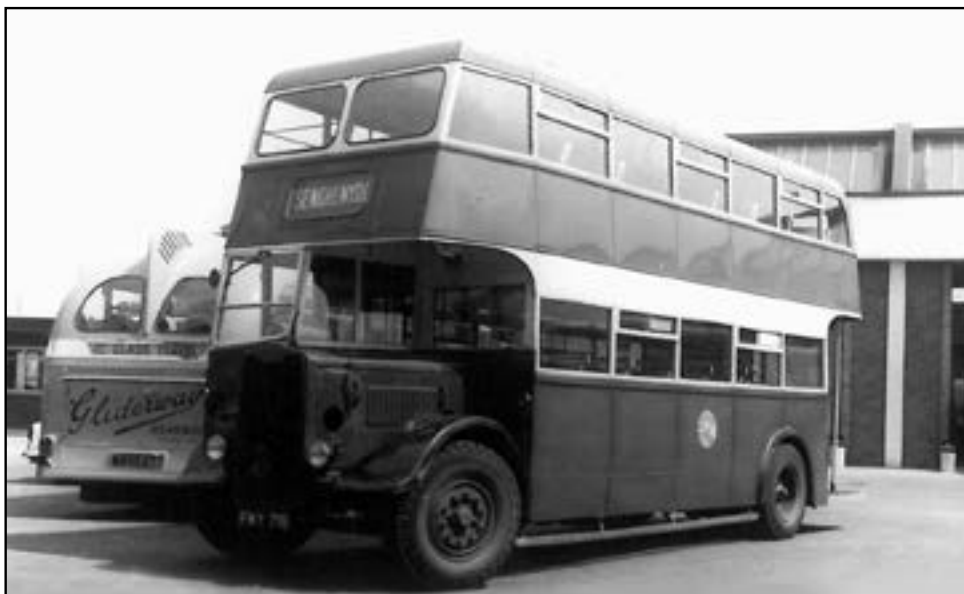
Roe-bodied Guy utility No. 18 (FNY 718) is seen at the garage. The date is not recorded but it was clearly after repainting in the new application of the livery and after rebuilding by the Council in 1956.
