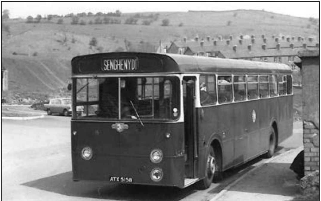
Another two Massey-bodied 36ft Leopards arrived in 1964. Number 15 (ATX 515B) is seen in 1966 at the turning circle in Senghenydd, with the Terraces in the background which were never reached during the Council's operations.
