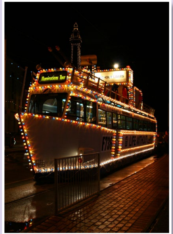
Illuminated cars HMS Blackpool, the Frigate created in 1965 and then restored and updated in 2003/4, and below the Trawler Cevic of 2001 sponsored by Fisherman's Friend. These new-generation illuminated cars use low-voltage lighting circuits for the bulbs instead of the traction-voltage series-wired arrangements of the past. (David Cole both)
