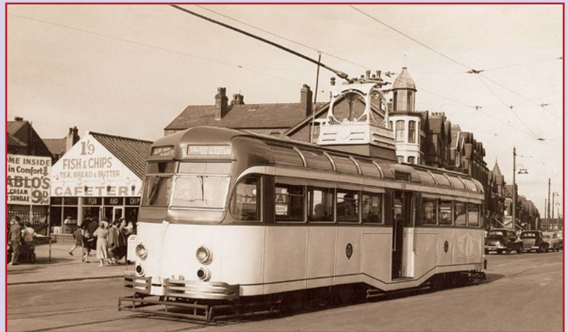
Number 208, now fitted with VAMBAC control, prepares to return to Talbot Square via Marton from Station Road in 1950. The base of the trolley tower clearly shows the modifications necessary to house the equipment. (JS King)
