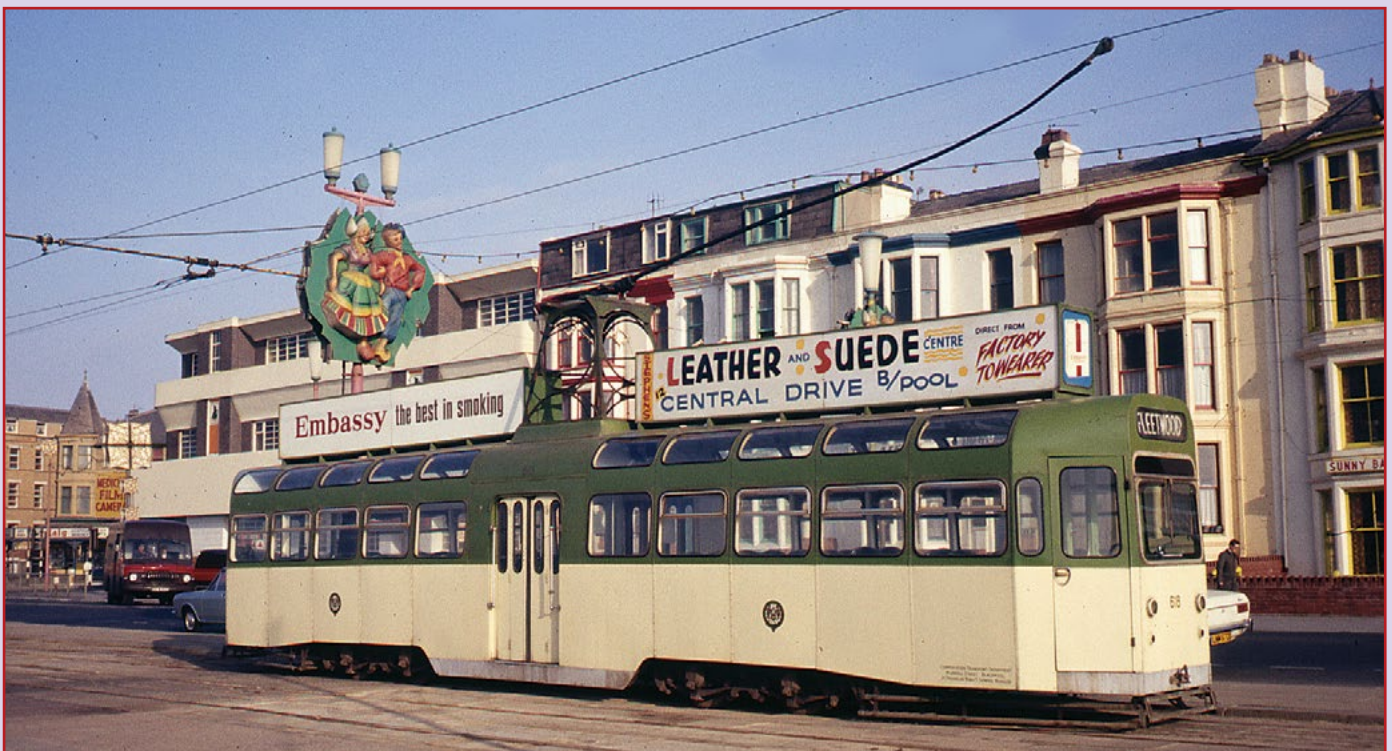
In 1968 number 618, below, formerly Railcoach 271, was the subject of what turned out to be an unsuccessful conversion whereby the seating capacity was increased from 48 to 56 after it was lengthened and fitted with tapered ends as seen here. It was decided to rebuild it to become the thirteenth one-man car, and as such it duly appeared numbered 13 in June 1976. It was the first of the class to be scrapped, in 1985. (STA)
