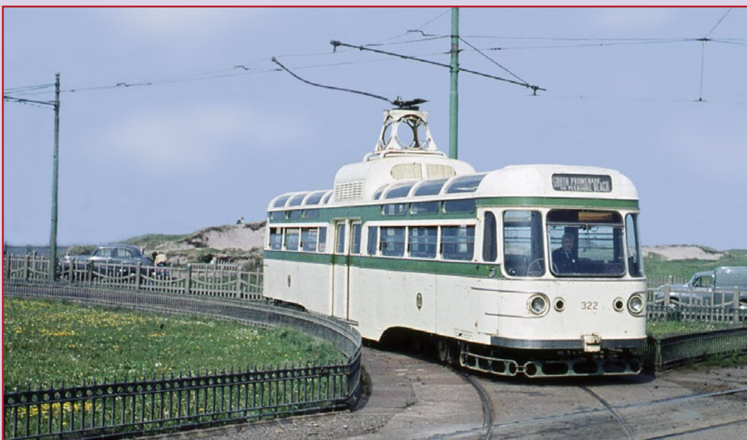
In better days Coronation 322 turns at Little Bispham loop. Twelve of the cars were given an extended life between 1964 and 1970 by the removal of the VAMBAC equipment and its replacement by controllers and resistances from withdrawn Railcoaches. Although it was a comedown it gave them six or seven extra years in revenue service. Three survive in preservation, number 304 restored with its original equipment at Rigby Road but owned by LTT, 660 as converted and the property of BTS and 663 in store with the LTT. (G Lumb)
