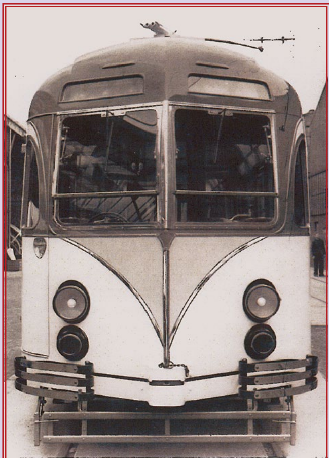
Front View of one of the Blackpool Tramcars. The Ends are Tapered, and Streamlining is Emphasised by Stainless Steel Mouldings
