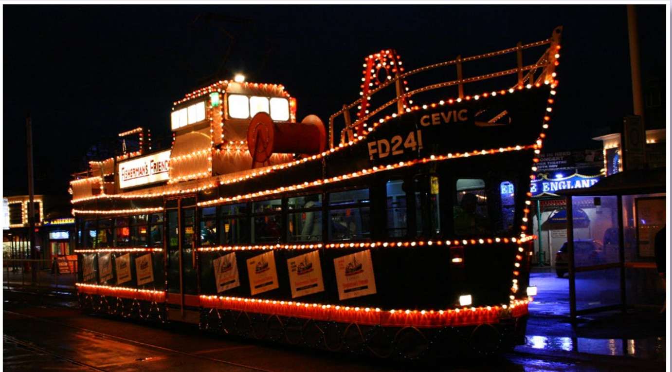
Illuminated cars HMS Blackpool, the Frigate created in 1965 and then restored and updated in 2003/4, and below the Trawler Cevic of 2001 sponsored by Fisherman's Friend. These new-generation illuminated cars use low-voltage lighting circuits for the bulbs instead of the traction-voltage series-wired arrangements of the past. (David Cole both)
