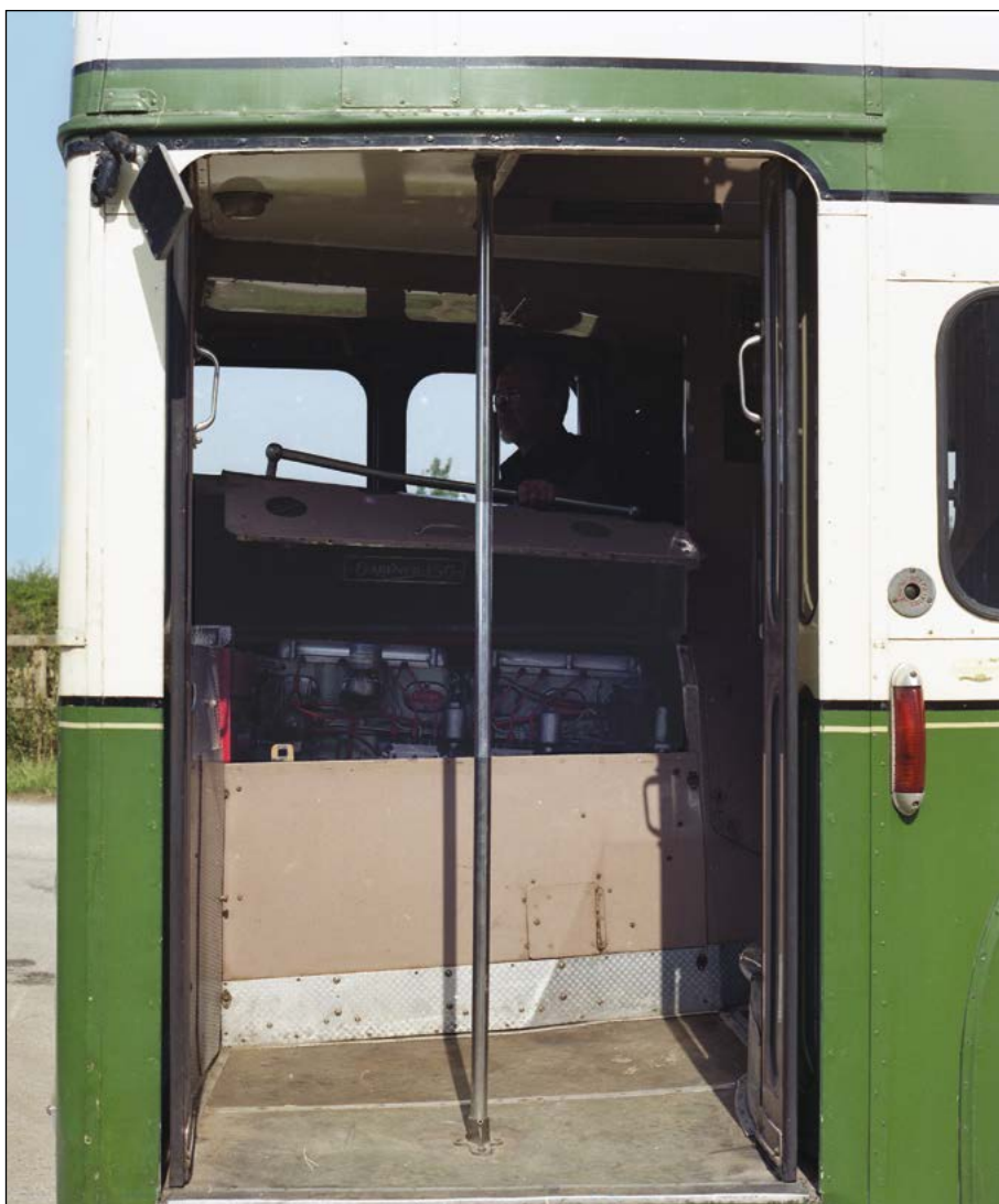
The nearside staircase location is evident in this three-quarter view of a preserved Wulfrunian, whilst the detail shot taken through the open door clearly shows the position of the Gardner 6LX engine on the platform, and the lightweight casing which covered it. (John Senior, both)
