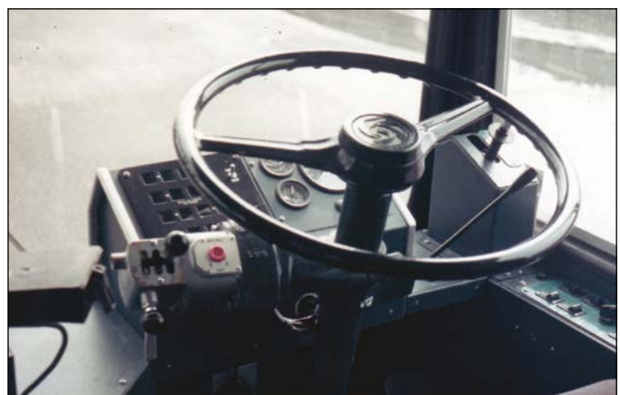
Brighton Corporation was the first operator in the south and west to have its own specification for its cab layout in place of the standard Leyland binnacle; this was on the later East Lincs bodies. Shown below is the cab of No. 67 (OYJ 67R), one of the two-door batch. (David Toy)
