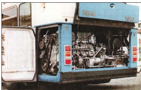
The Atlantean bustle disappeared on the new Olympian and a two-piece hinged engine door was fitted, supported by gas struts, greatly improving the appearance of the rear of the bus bodywork. Access to the sides of the engine compartment was by two doors, and under trays were also fitted. (Leyland)
