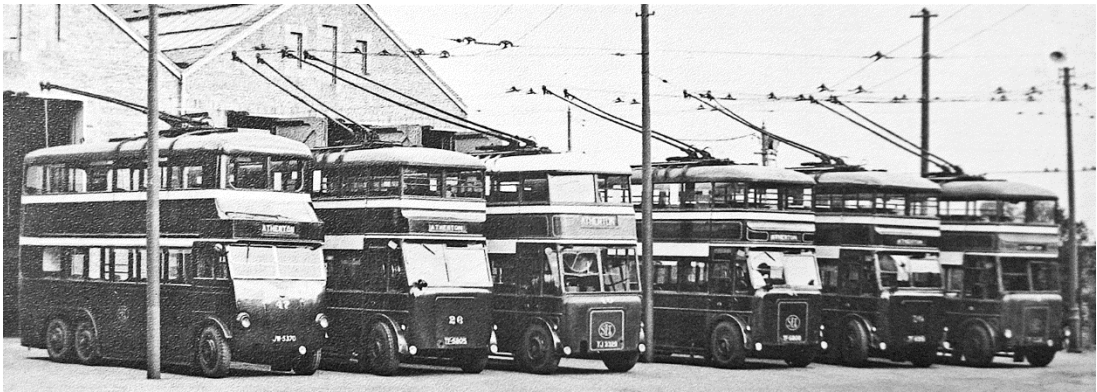
Taken outside the garage, this line up shows the different steps in the piano-front of the BTXs (26 second from left and three others fourth, fifth and sixth) and the BTs (40, third from left). Second-hand ex-Guy demonstrator, 47, is on the left
