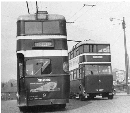
Number 6 with the flat front panel. The rear view of number 9 shows the absence of an upper-deck emergency door, the revised rear platform window fitted on rebuild and the St Helens licence number at the lower left of the rear panel.
