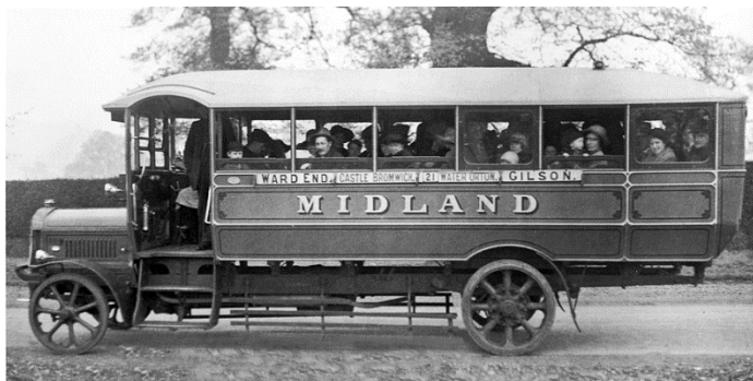
This BMMO (Midland Red) body, for which LUT bought drawings and a licence, was the basis of the BCLE bodies built for LUT one of which is pictured below.
