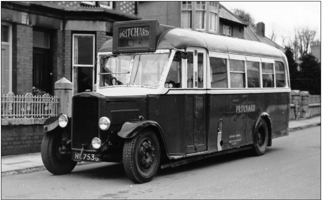
Leyland KP22 Cub HL 7538 was already 13 years old when West Riding sold it to Pritchard of Newborough in June 1949. Its Roe bus bodywork had originally held 20 passengers but at some point during the Second World War had been 'upseated' to carry 26. The vehicle is seen in Llangefni on Pritchard's market-day service in November 1966 when it had already passed its 30th birthday. It continued in service until the following year and was then sold to Hollis of Queensferry for use on 'heritage' work. It is now preserved in Pritchard's blue and cream livery. (Nick Craig)
