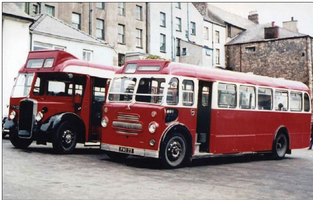
Here we see Express Motors' two forward entrance Bristol 'L types' side by side in Caernarvon. FFM 524 was a 35-seat L6A half-cab, modified by its original owner Crosville before passing to Express in February 1967. The modifications to FMO 23, a 39-seat LL5G had been made by Thames Valley and included a full-front as well as the repositioned entrance. (JT Williams Collection)
