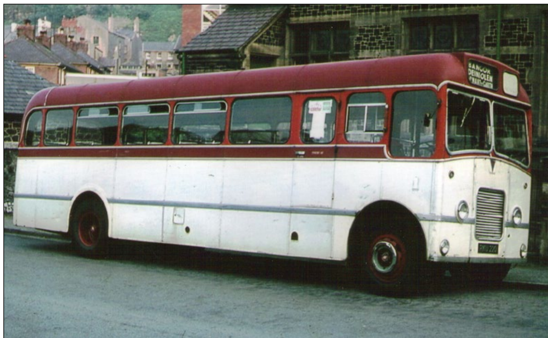
AEC Regal III RKU 220 was new to an unidentified Bradford operator in 1948 as a half-cab coach. By 1958 it was owned by Rhind of Wakefield and they decided to rebody the vehicle as a fully-fronted 39-seat bus to Plaxton's new Highway design. In January 1964 the Regal was sold to Deiniolen Motors and is seen here in Bangor on a short working of their Dinorwic service. (Vic Nutton)
