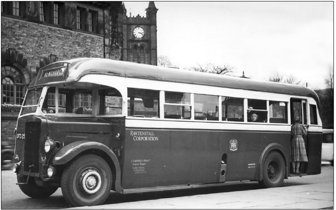
Number 46, a Leyland TS8c, with Leyland body was one of two similar buses supplied in 1938 and was still giving service when photographed above in Rawtenstall in April 1954. A similar vehicle supplied in 1939 and numbered 50 has been preserved and regularly appears at rallies, as seen below. The deep header tank for the Autovac on the bulkhead confirms that the vehicle still has its torque-converter, but the preserved example lost its unit in exchange for a conventional gearbox some time before withdrawal. ( RM upper, JAS lower )
