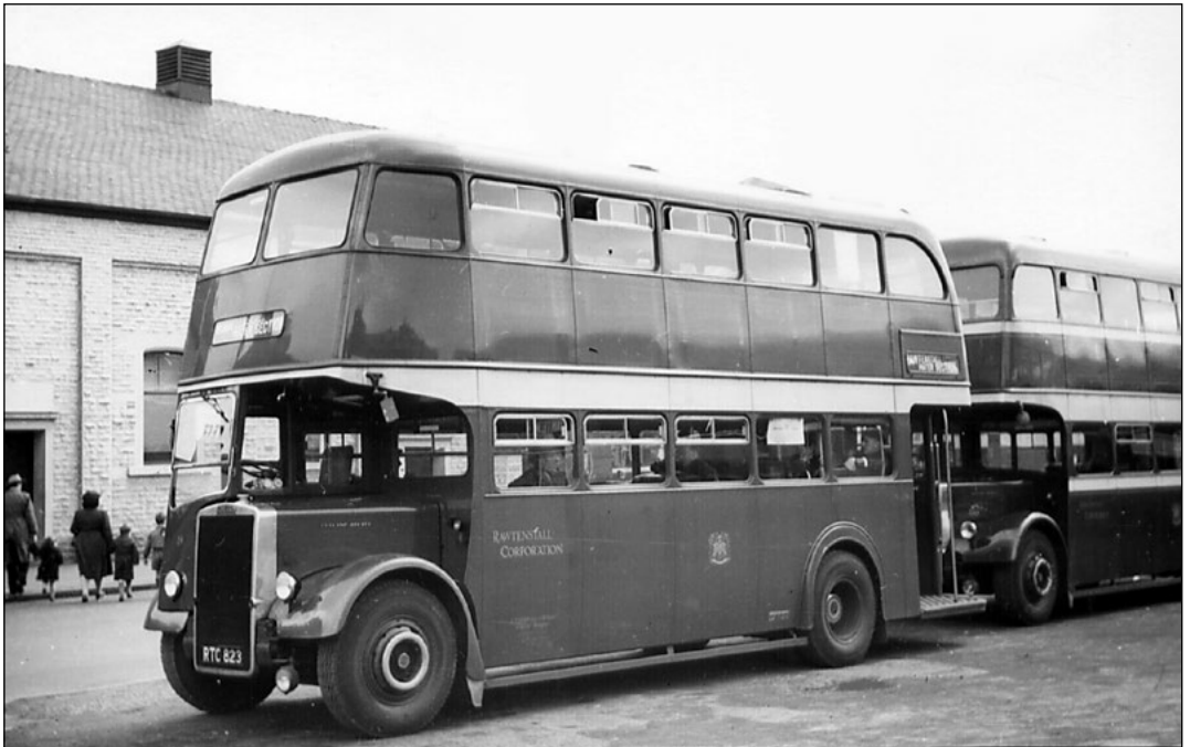
The last Leyland-bodied vehicles arrived in 1953, after which the company ceased manufacture of bus bodywork. Number 18 pictured above en route to Bacup in October 1964 illustrates the final style of Leyland double-deck bodywork, with window pans radiused at both top and bottom. The lower photograph shows sister vehicle No. 19 in April 1954 in an experimental livery incorporating only one cream band. Happily, this simpler livery was not adopted! (RM)
