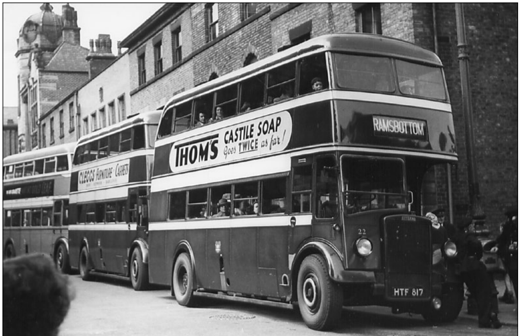
The first double-deckers to be purchased by Ramsbottom arrived in 1947 numbered 20-25 and were Leyland-bodied Leyland PD2/1 models. Number 22 is shown in Bury in April 1954, with another from the same batch behind, and also a Bury Corporation double-decker. (RM)
