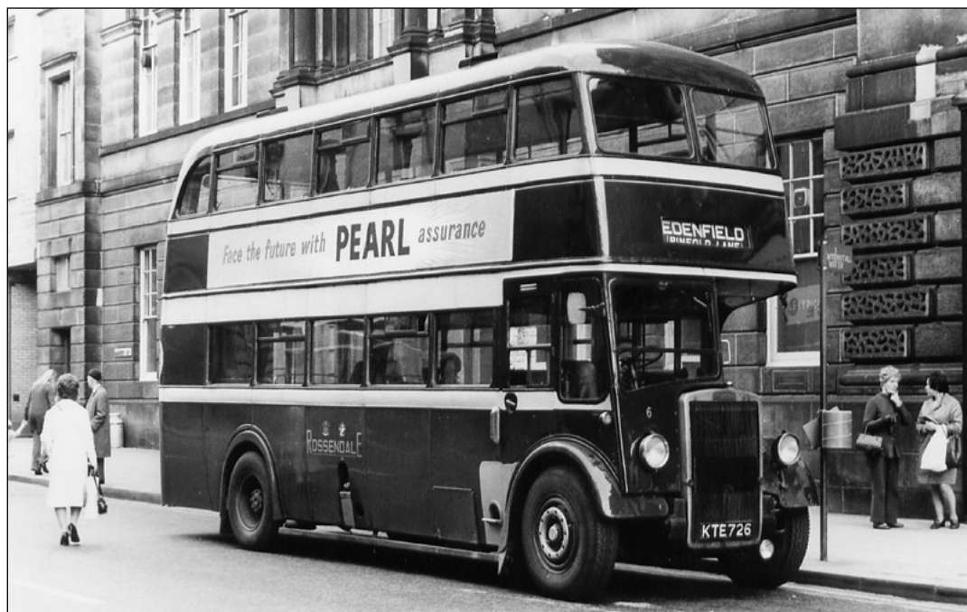
Former Rawtenstall No. 6, a 1949 Leyland PD2 with Leyland body is shown in Bury awaiting departure to Edenfield in May 1971. On the earlier PD1 model the dash panel covered the offside front wing. (BD)
