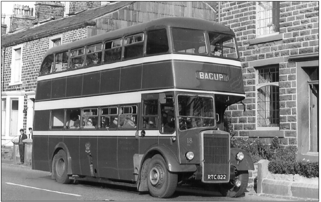
The last Leyland-bodied vehicles arrived in 1953, after which the company ceased manufacture of bus bodywork. Number 18 pictured above en route to Bacup in October 1964 illustrates the final style of Leyland double-deck bodywork, with window pans radiused at both top and bottom. The lower photograph shows sister vehicle No. 19 in April 1954 in an experimental livery incorporating only one cream band. Happily, this simpler livery was not adopted! (RM)
