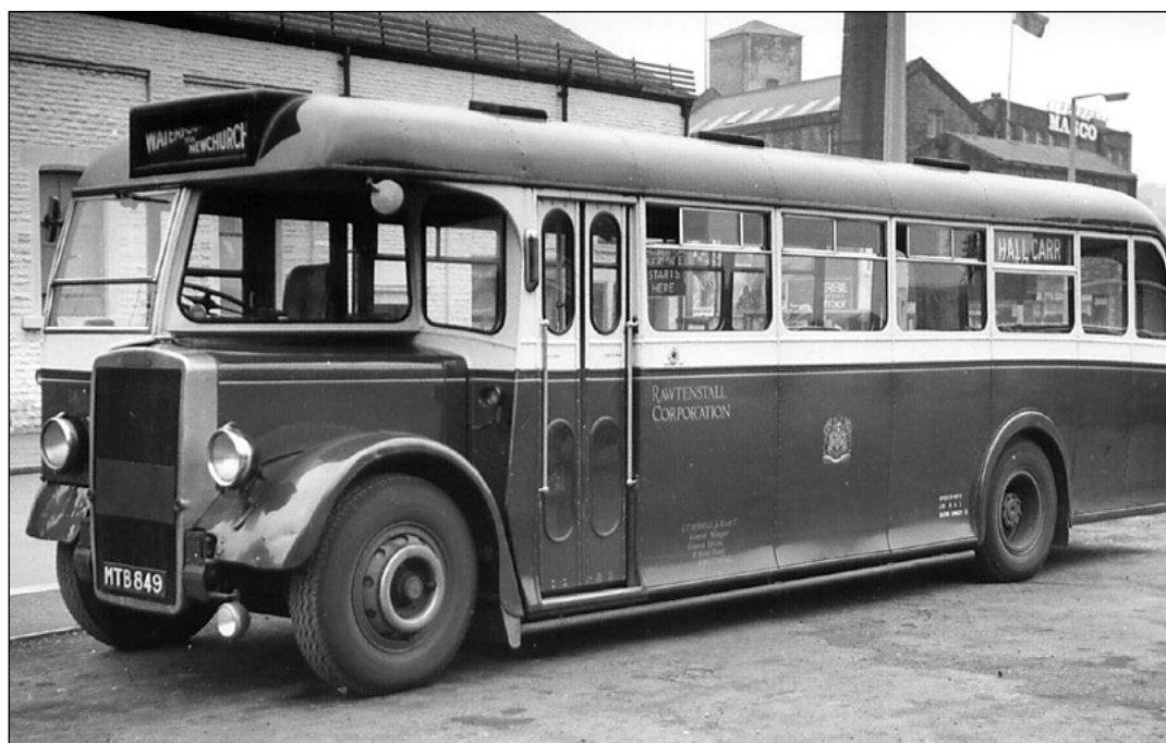
Above: The first postwar intake of single-deckers for Rawtenstall arrived in 1949 and were two ELCB-bodied Leyland PS1 Tigers, Nos. 53/54, the first of which is shown in Rawtenstall in August 1953. (RM)
