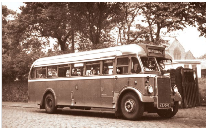
Haslingden's first post-war single-deckers, numbered 1-4, comprised two Leyland PS1 and two PS2 models, delivered in 1949. All four had bodies by HV Burlingham of Blackpool, and No. 2 is shown in Haslingden in June 1951. This bus has been preserved in Haslingden livery and often appears at rallies. (RM)
