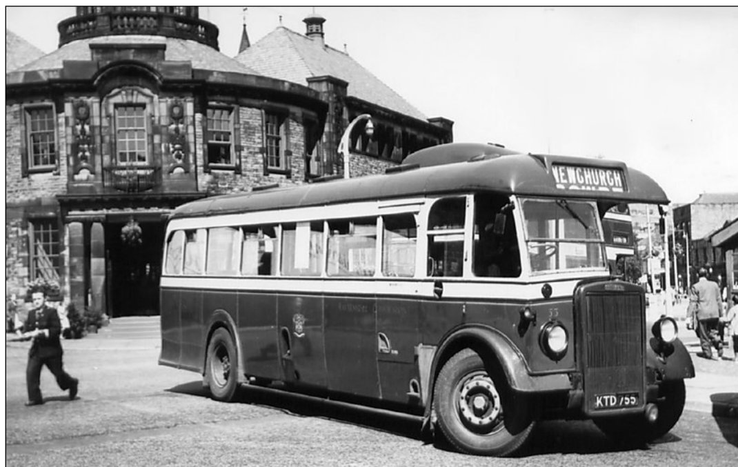
Above: The first postwar intake of single-deckers for Rawtenstall arrived in 1949 and were two ELCB-bodied Leyland PS1 Tigers, Nos. 53/54, the first of which is shown in Rawtenstall in August 1953. (RM)
