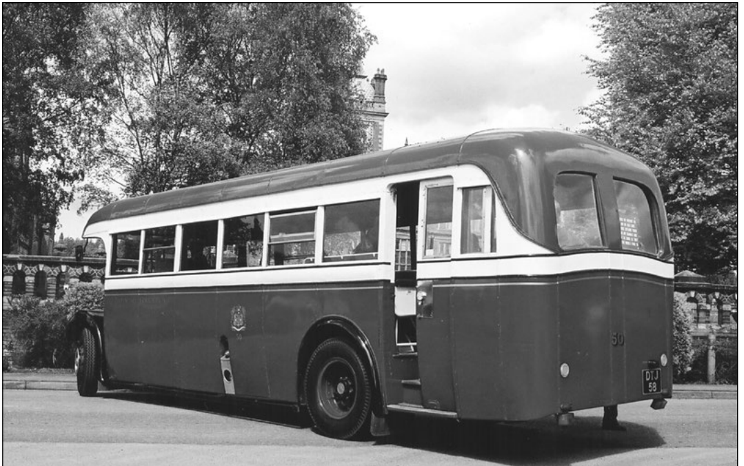
Number 46, a Leyland TS8c, with Leyland body was one of two similar buses supplied in 1938 and was still giving service when photographed above in Rawtenstall in April 1954. A similar vehicle supplied in 1939 and numbered 50 has been preserved and regularly appears at rallies, as seen below. The deep header tank for the Autovac on the bulkhead confirms that the vehicle still has its torque-converter, but the preserved example lost its unit in exchange for a conventional gearbox some time before withdrawal. ( RM upper, JAS lower )
