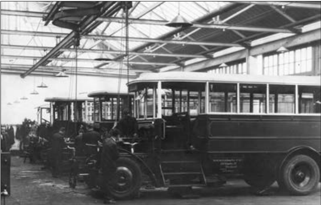
One of North Western's striking Brush-bodied Tilling Stevens petrol-electric buses is seen in Mersey Square soon after delivery in 1925. It is operating on the former British route to Cheadle. The petrol engine drove a dynamo which produced the electricity for an electric motor which powered the vehicle. Remarkably, one of these fascinating vehicles survives, fully restored, in the Museum of Transport in Boyle Street, Manchester. After withdrawal many passed to fairground showmen who were able to use the dynamo's output to power their attractions. The scene below also dates from the mid-1920s and shows a selection of buses undergoing maintenance and repair in North Western's Charles Street workshops. (STA both)
