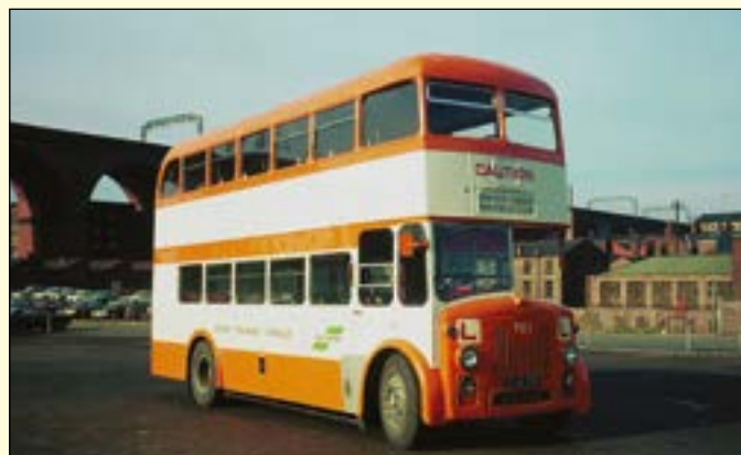
PJA 918, formerly number 348, became a driver trainer as seen here, and was numbered TV.1. Such vehicles were retained by virtue of their non-automatic gearboxes, as drivers passed on automatics were restricted to driving vehicles with that type of transmission. (STA)
