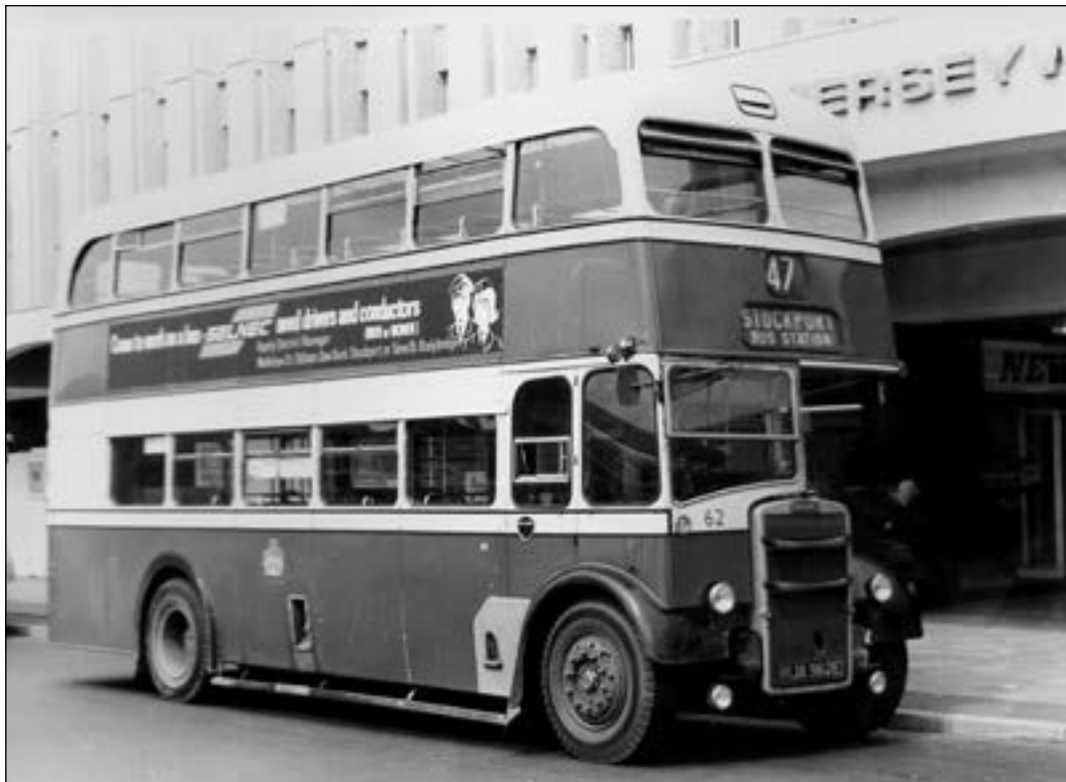
No less than 30 of the by-now standard Leyland/East Lancs design were taken into stock in 1967. There were in fact two batches this year; Nos. 41-55 (HJA 941-55E) being standard products, but Nos. 56-70 (HJA 956-70E) actually had bodies built in Sheffield by Neepsend to East Lancs design, both companies at the time being part of the Craven group. Notice the indicators, now at the front above the cab, and the advert on No. 62; although still in Corporation livery the bus belongs to SELNEC PTE and staff recruitment is necessary. (AEJ: BD)
