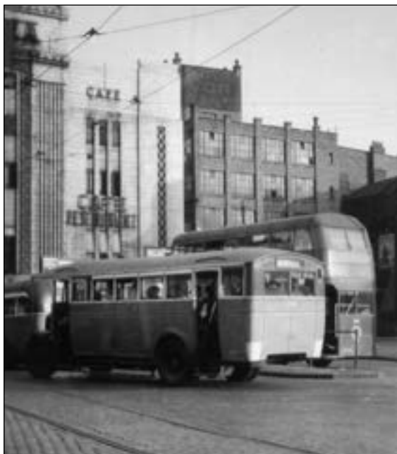
Wartime Mersey Square, with two views of PLSC Lion number 124, the Cravens body recognisable by its shallow windows, and Guy Utility 216 in wartime garb but with matt paint on the roof contrasting with the sheen of the body panels. Note that both vehicles display the garter logo on the rear panels whilst the Lion also has two white warning patches. (Maurice Marshall collection courtesy Chris Heaps)
