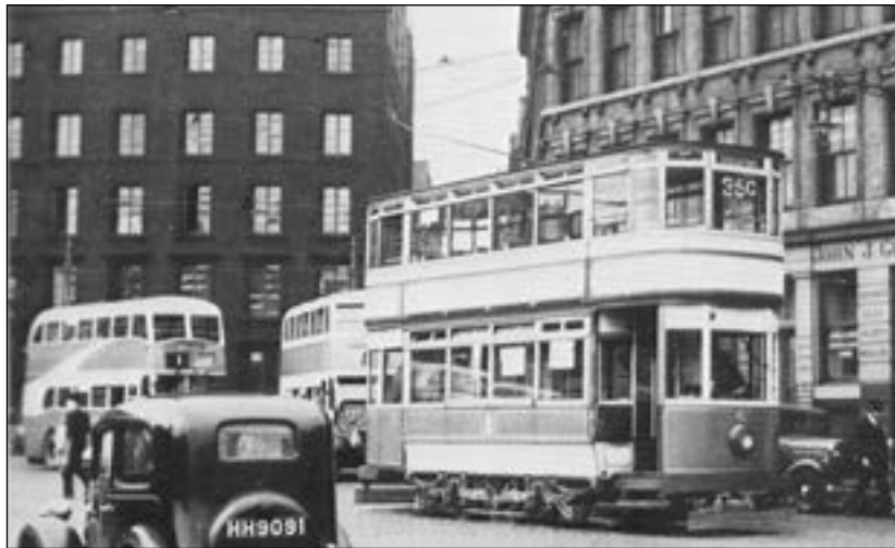
Manchester's Albert Square, terminus of the 35C, and car 6 stands with the Corporation's buses. The new Leyland double-decker is on the Limited Stop service to Gatley where once Stockport's trams terminated, of course. Tram number 6 was an entirely home-made production by Stockport, assembled from spare parts and completed by bespoke bits to fill the gaps, and fitted to a truck which was also spare. Waste not want not – it was this policy of re-utilisation of assets which made the Department so efficient. (MMC)
