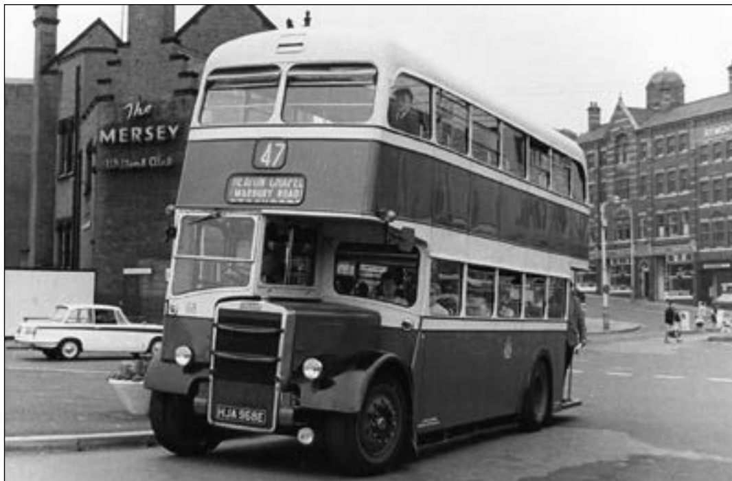
No less than 30 of the by-now standard Leyland/East Lancs design were taken into stock in 1967. There were in fact two batches this year; Nos. 41-55 (HJA 941-55E) being standard products, but Nos. 56-70 (HJA 956-70E) actually had bodies built in Sheffield by Neepsend to East Lancs design, both companies at the time being part of the Craven group. Notice the indicators, now at the front above the cab, and the advert on No. 62; although still in Corporation livery the bus belongs to SELNEC PTE and staff recruitment is necessary. (AEJ: BD)
