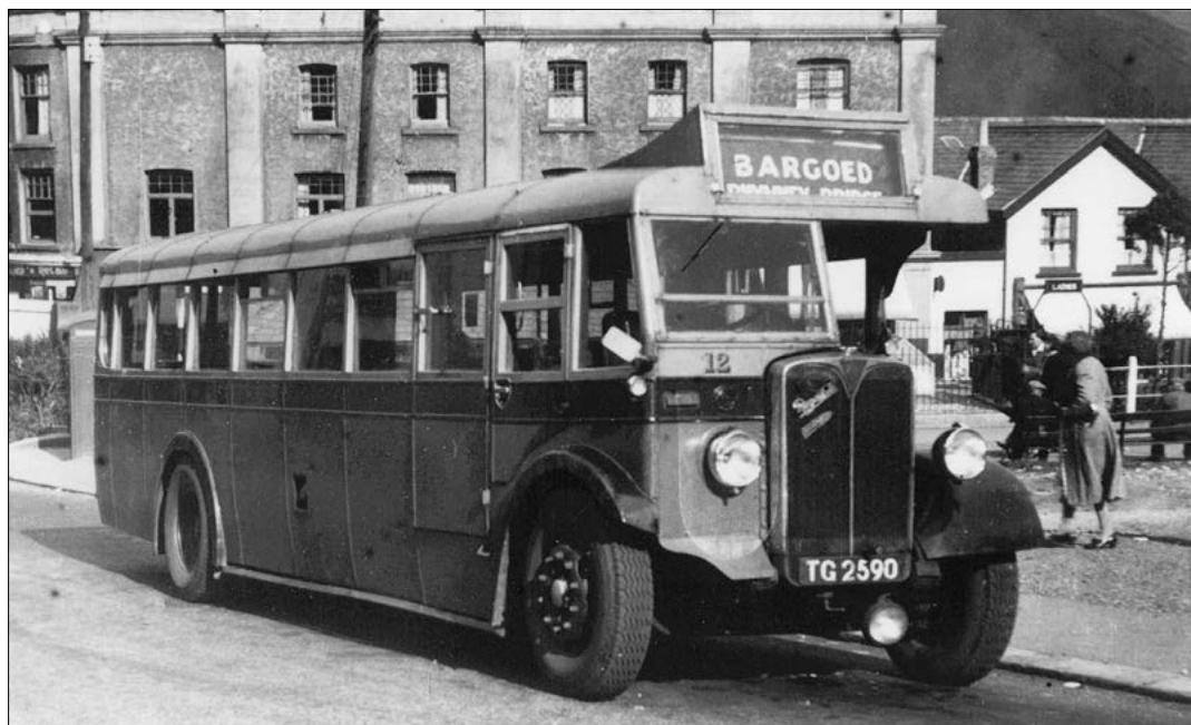
One of a pair of AEC Regals delivered in 1931 was No.12 (TG 2590) which was delicensed and then rebuilt between 1947 and 1949. This picture was taken in 1950 and shows it at Bargoed.
