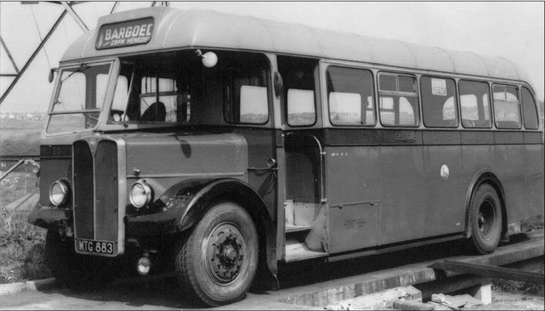
The first vehicles bodied for the Council by Longwell Green arrived in 1953. No.12, later 10 (MTG883), on AEC Regal III chassis, is seen at the garage at Tiryberth in 1967. In 1954 the last two vertical-engined single-deckers arrived. No.2, later 12, was one of the last AEC Regal III chassis supplied for the home market. The nearside of its Longwell Green bodywork is shown clearly at the back of the garage in 1966.
