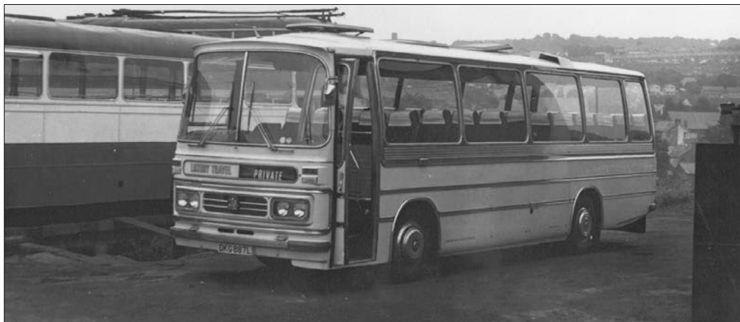
One of the shortest lived of the Council's vehicles was No.102 (DKG 887L), a Bedford YRQ with Duple C45F body which was designed for private hire work and was delivered in April 1973 in an all over cream livery. It is seen here at Tirryberth in September of that year, but had gone by December.
