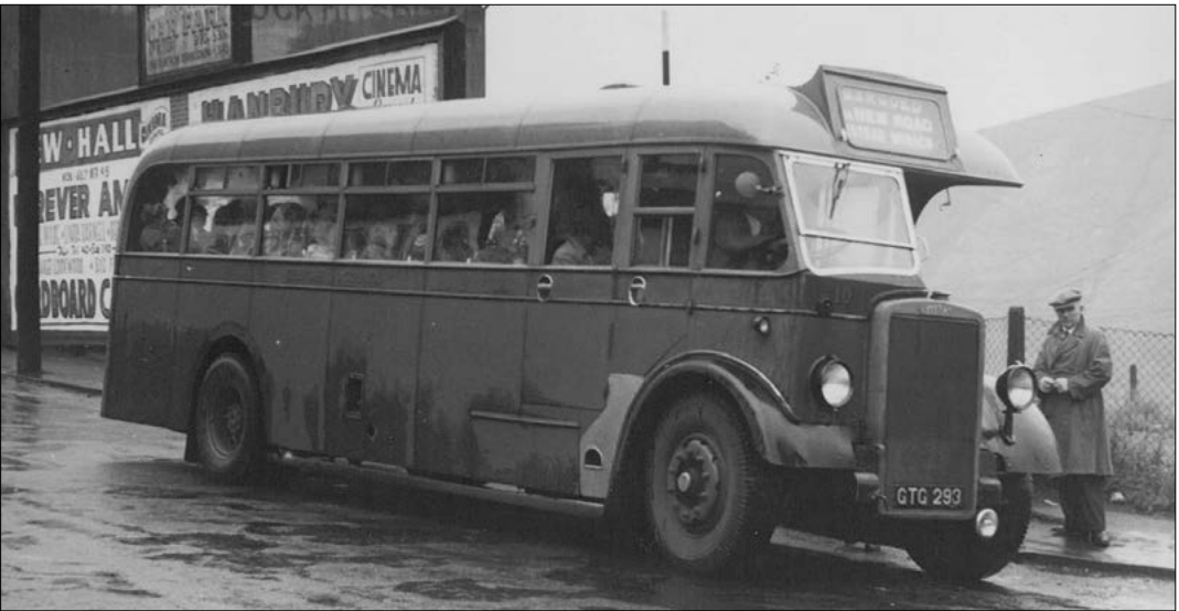
Three Leylands on PS1/1 chassis with Willowbrook bodies arrived in 1947. No.10 (GTG293) is seen in Bargoed on Roy Marshall's first trip to the area, in 1949.
