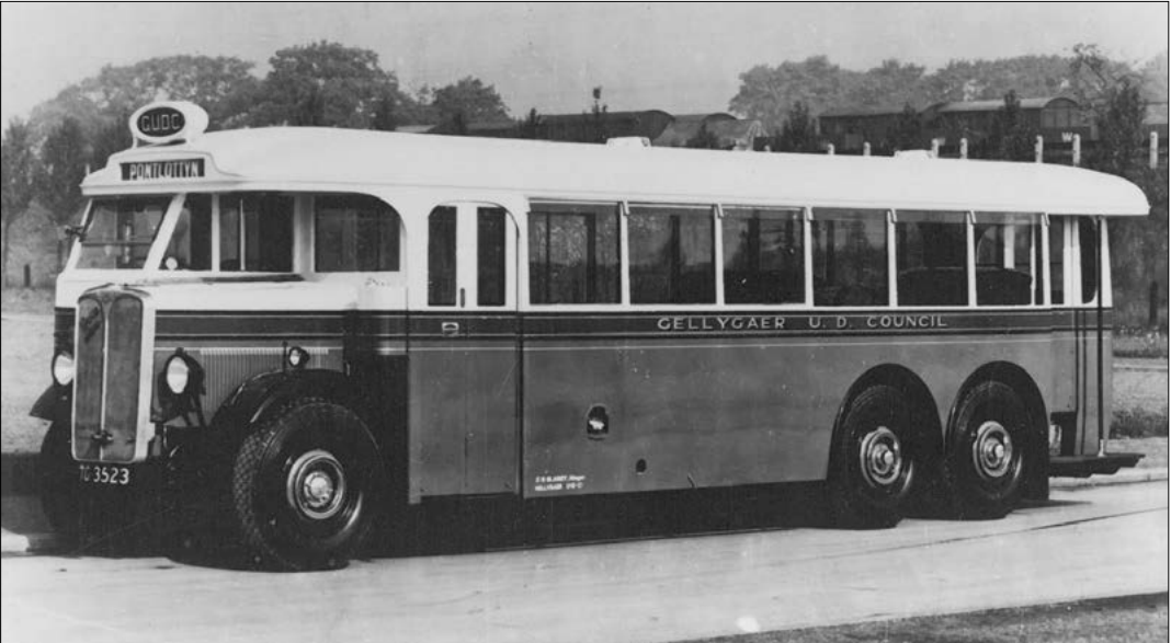
Weymann-bodied AEC Renown delivered in 1932, is seen before conversion to rear-entrance only in 1934.
