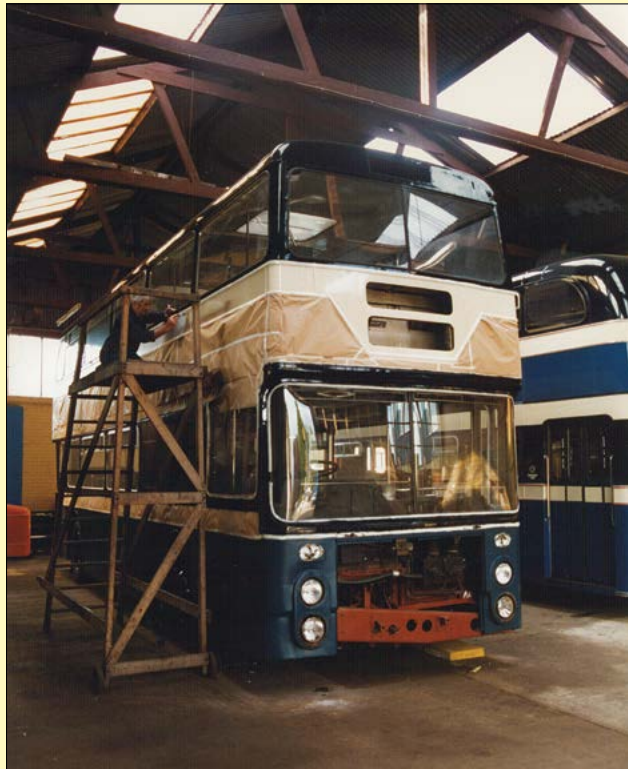
Inside the shed in 1996, before rebuilding, Atlantean No. 120 is at the repainting stage with coachbuilder Tony Clark applying cream paint between the decks. All refurbished vehicles were out shipped to the usual very high Delaine standard. Also in the shed is preserved PD2 No. 50.
