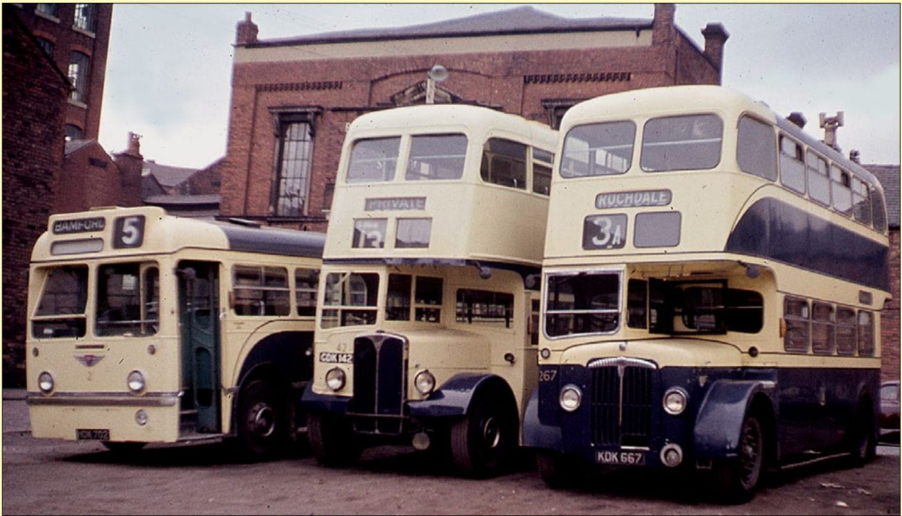
Three Rochdale vehicles showing the original and later liveries. Number 2, left, is an AEC Reliance, No.42 an AEC Regent III and 267 a Daimler CVG6. All three carry bodywork by Weymann and the difference in body width between the 7ft 6in wide Regent and the 8ft Daimler is clearly seen. With the exception of five Reliances from Salford in the Central Division all the AECs SELNEC inherited pre- NWRC happened to be in fleets in the Northern Division. Joe Franklin, Rochdale's then manager, had been Salford's engineer under Charles Baroth and later moved to take charge at Blackpool. (APY)
