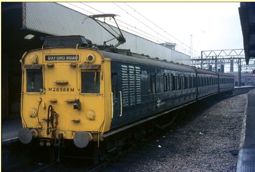
3-car EMU built by Metropolitan Cammell Carriage & Wagon Co. for the electrification of the Manchester South Junction and Altrincham Railway. The electric service started on 11th May 1931, with 6-car trains being operated in the peak. During World War II 7-car trains were tried but did not prove satisfactory in blackout conditions. Twenty-two sets were built and this one, M28588M, was 39 years old when photographed in the bay platform at Oxford Road. (DSH)
