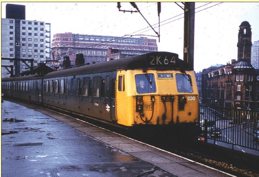
A 4-car Type AM4 EMU arriving on Platform 13 at Piccadilly Station with an Altrincham-Crewe working. In 1971 the MSJA was converted to 25 kV AC operation, although many of the overhead gantries and wiring were retained, only being replaced in the major Matrolink upgrade of 2009. The new AC units were slower than their predecessor DC units on the Altrincham line, but linking services round the south side of Manchester probably meant that overall journey times were little changed. (APY)
