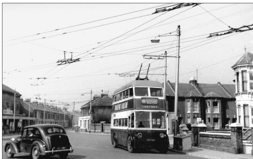
Post-war BUT No. 304, ERV 929, speeds across the northern leg of Bradford Junction in April 1963. By this time the wiring into Rugby Road from Bradford Road has been removed. The ears where running wire has been spliced in may be seen. (ADP)
