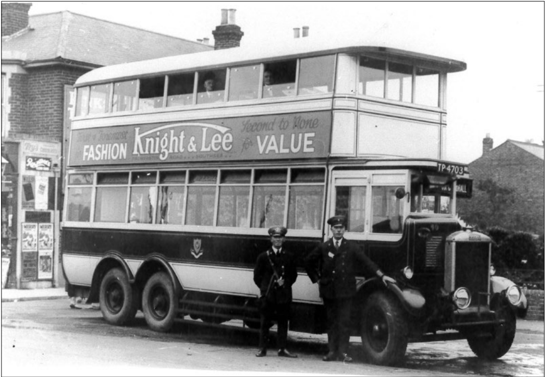
The first high-capacity double-deckers were 14 Karrier WL6/2, with seats for 60. Number 40, TP 4703, was the first and had a Brush body as did seven more delivered in 1927. It is seen at the Cosham Railway Station terminus opposite Cosham Compound where the tram services terminated. (RM)
