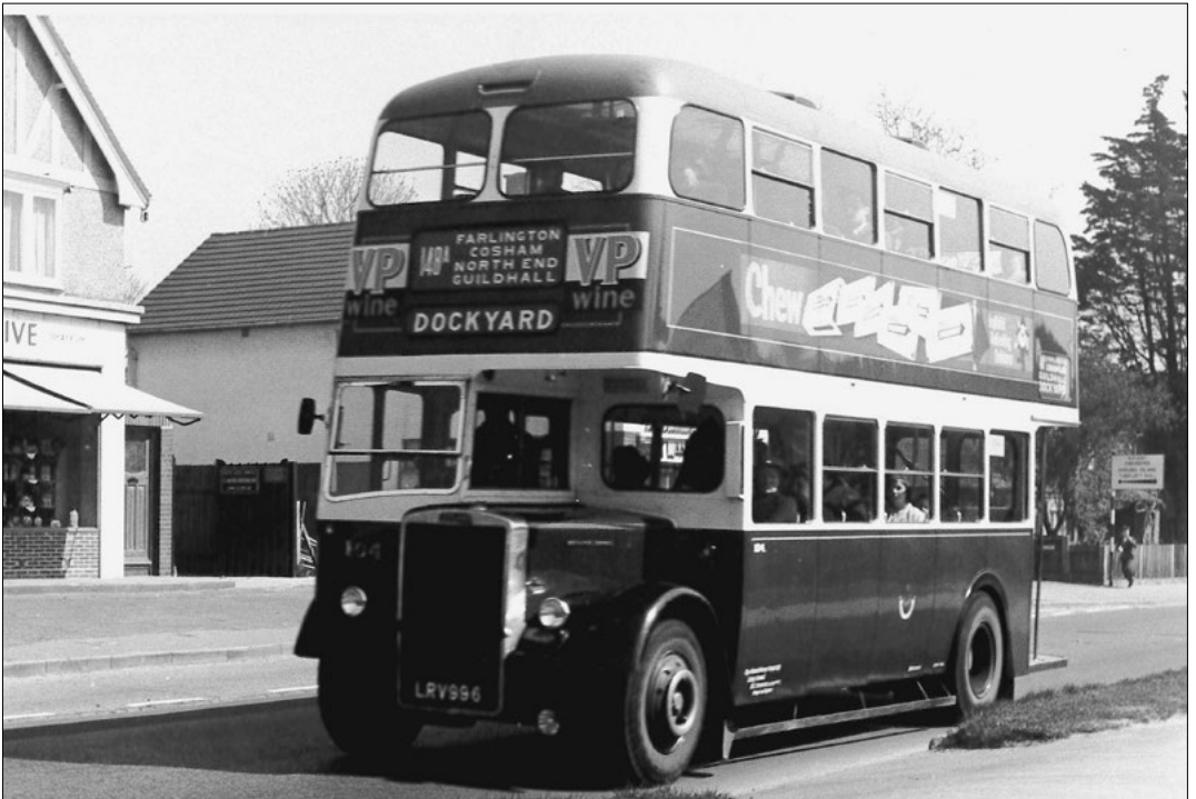
In 1956 Portsmouth turned to Metro-Cammell as the supplier of its bus bodies for double-deckers and this was to remain the case for the next ten years. Twenty five Leyland PD2/12s were involved in this order. With two Isle of Wight paddle steamers in the background, No. 97, LRV 989, waits on the 148B stand at the Dockyard. The suffix letter of the route number indicated the route and terminus in Leigh Park. Note the provision still of a semaphore arm for signalling. Returning from that location is another Leyland PD2/12, number 104, this time operating on service 148A and seen at Bedhampton.
