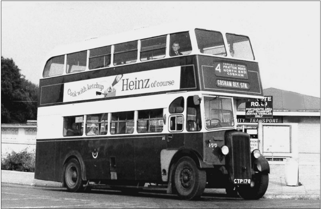
An off-side view of No. 177 at South Parade Pier after repainting with a white roof (a variation to the fleet livery re-introduced in 1960) and the fitment of flashing indicators.
