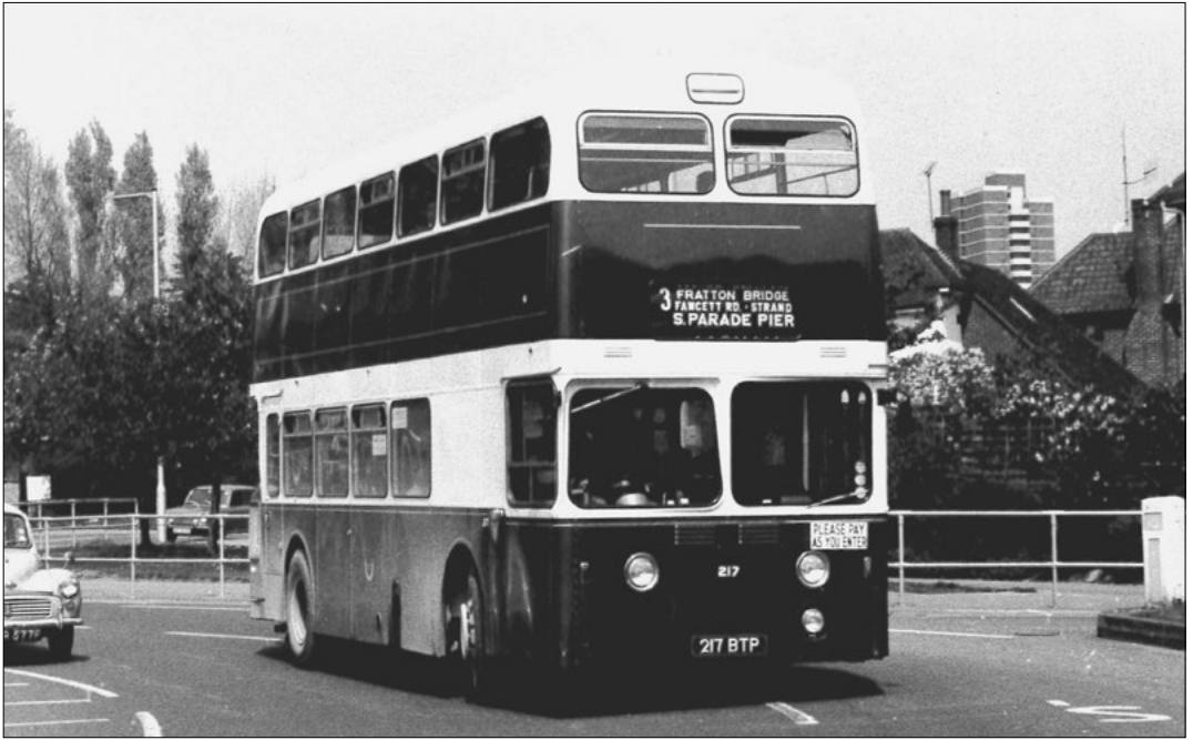
One-man-operation, using Leyland Atlanteans, resulted in the vehicles having to be modified for this purpose and No. 217, 217 BTP, which was rebuilt in 1970, had its destination display reduced as a result. It is seen negotiating the roundabout at Spur Road, Cosham. (ABC)
