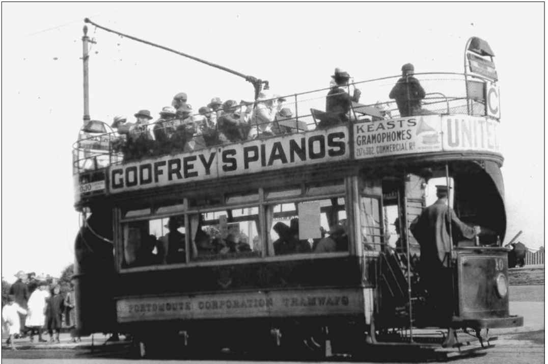
The motorman awaits the bell at South Parade Pier. The restricted visibility to the left as a result of reversed stairs being fitted to these trams is clearly apparent in this picture. Number 10 is operating on route C. (ADP)
