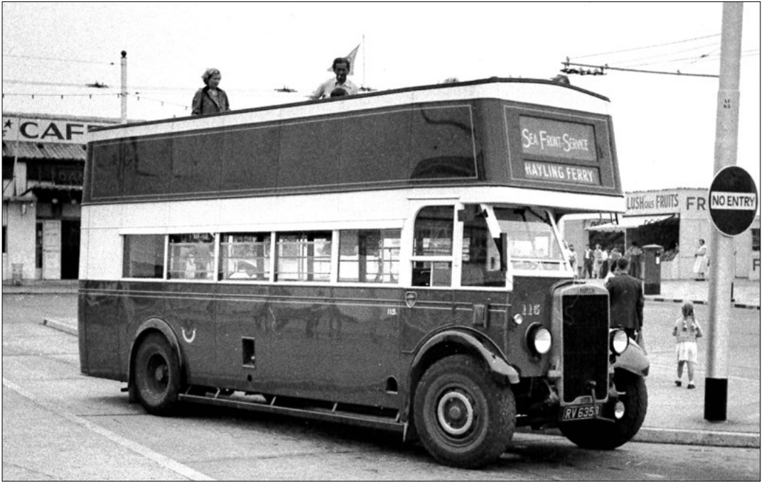
English Electric-bodied Leyland TD4 No. 115, RV 6358, was the first of 12 similar buses delivered in 1935 and was the first to be converted to open-top in 1953. Five years after conversion it was renumbered 5. (STA)
