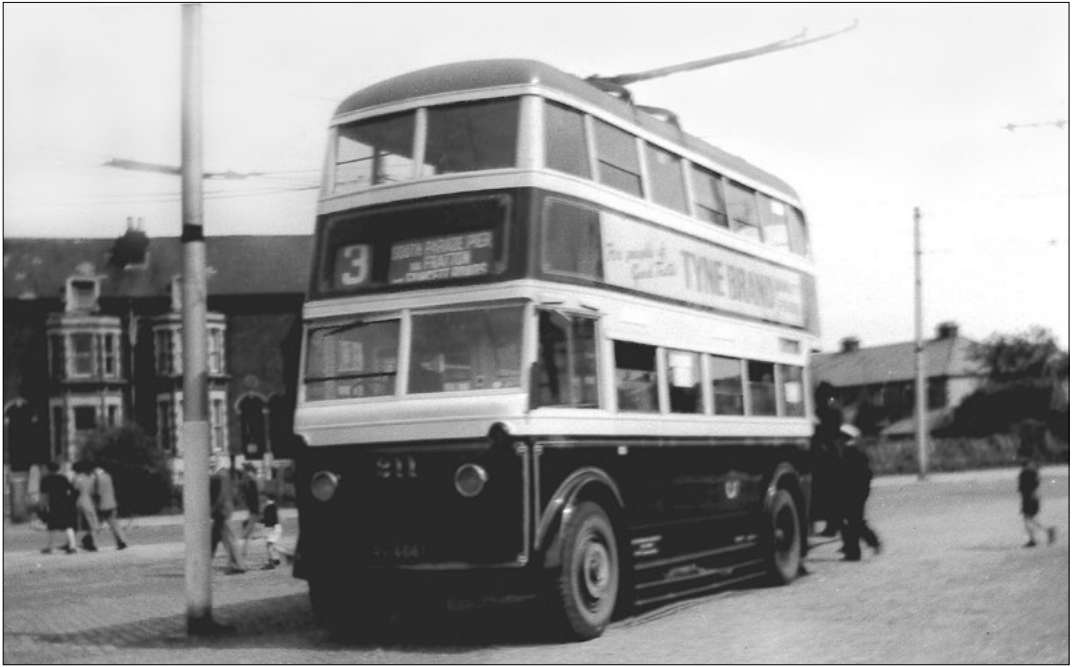
The body on Karrier E4 No. 211 was by Metro-Cammell, and although built with five-bay construction, tended to look more ancient than the English Electric example. Having arrived at Cosham Compound in early post-war days the destination screen had already been changed for the next journey to South Parade Pier (pre-war screens are still carried). (ADP)
