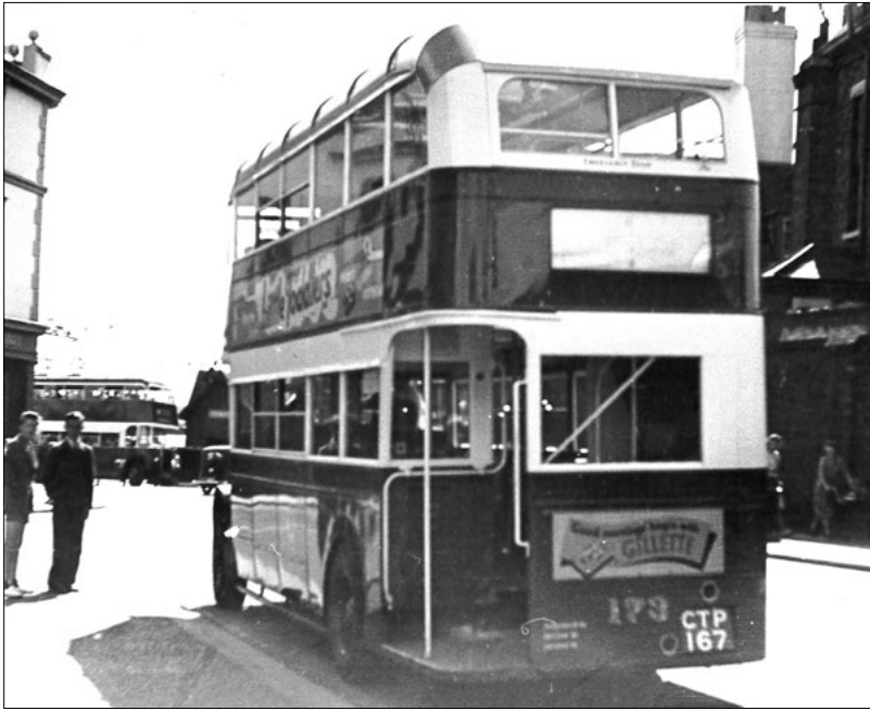
The only double-deckers to be delivered during the war were nine Daimler CWA6s, also with Duple bodies. This rear view of No. 173, CTP 167, clearly shows the angular lines of the roof of a Utility body. (ABC)
