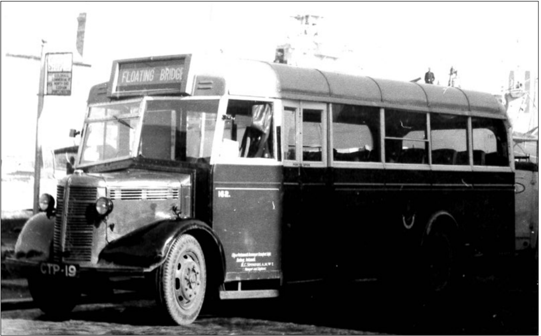
The second wartime delivery, No. 162, CTP 19 another Bedford OWB, was fitted with Mulliner bodywork. It is seen at the Floating Bridge terminus of the 145 service, which operated as a shuttle to Guildhall on Sunday mornings.
