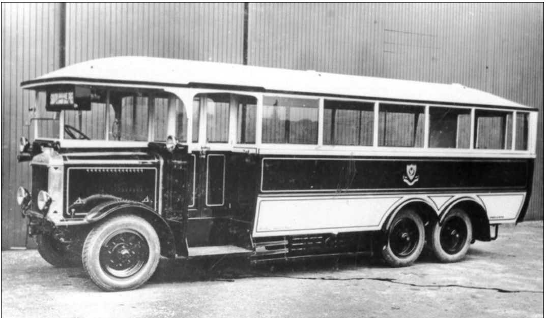
One of the pair of Karrier CL6s, also with Ransomes bodies, number 38, TP 4812, which were taken into the fleet in 1927 and seated 39. (RM)
