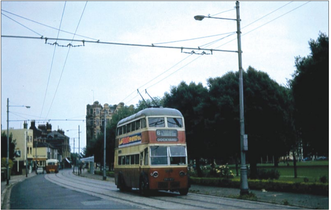
Pictured during the last few weeks of service No. 313, delivered in 1950 and now to be found in preservation at the East Anglia Transport Museum, travels along Southsea Terrace where tram lines, disused for 27 years, remained with only tar covering the metals. This was one of 15 BUT 9611Ts with Burlingham bodies which were Portsmouth's only post-war trolleybuses.
