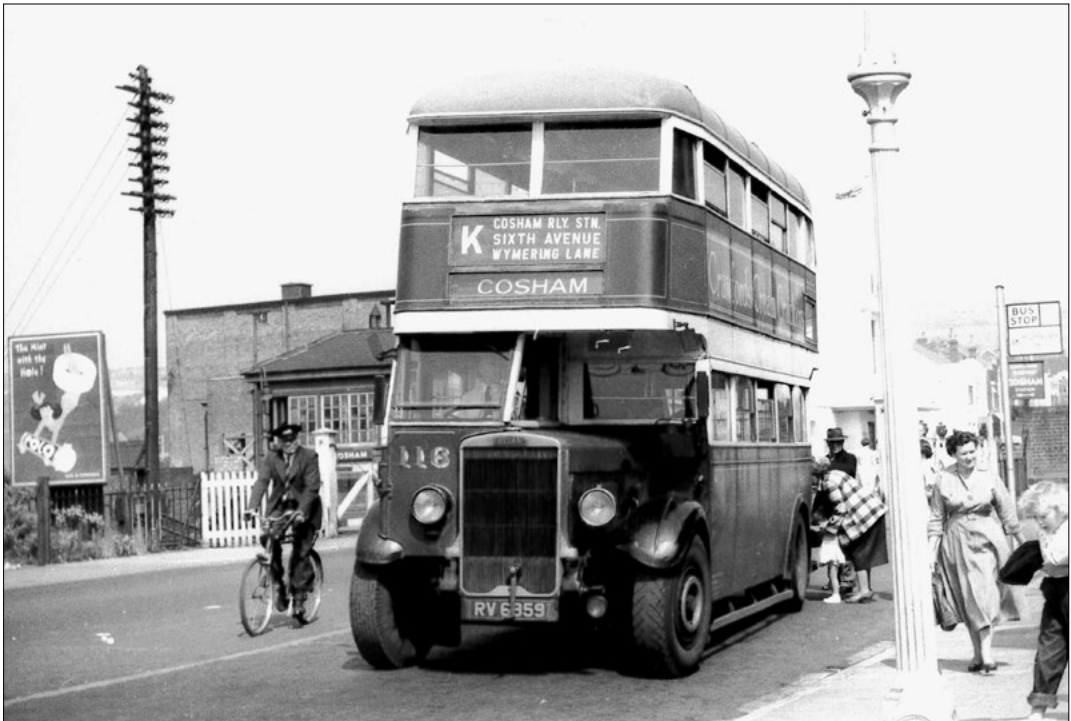
Two views at Cosham Railway Station of the J and the K which also allows a comparison of bodywork on the Leyland version (on No. 130 above) and English Electric one (on No. 116 below) on these 1935 Leyland TD4s. Space does not permit an explanation of the rather complicated history of these two services which strictly speaking were not a pair. (RM both)
