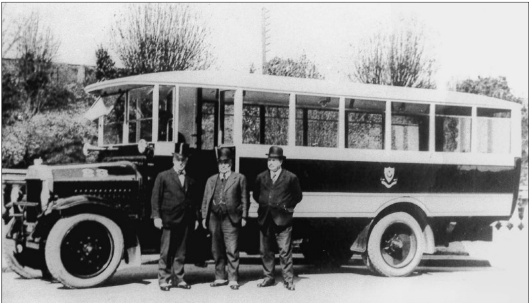
The formality of the officials would tend to suggest that this picture from 1925 of No. 23, TP 751, was taken during the hand-over of the first of 12 all-Dennis single-deckers. When new these 26-seat buses were used with a driver only. (RM)
