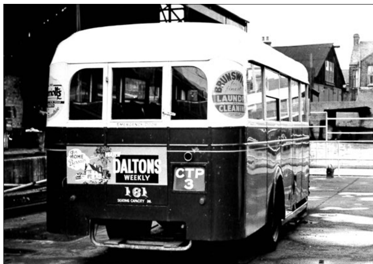
The first bus to be delivered during the war was No. 161, CTP 3, a Bedford OVB with a Duple 32-seat body. It arrived painted in an all-over brown livery but is seen here parked at Eastney depot in the final form of livery it carried. Note the carrier for the spare wheel.
